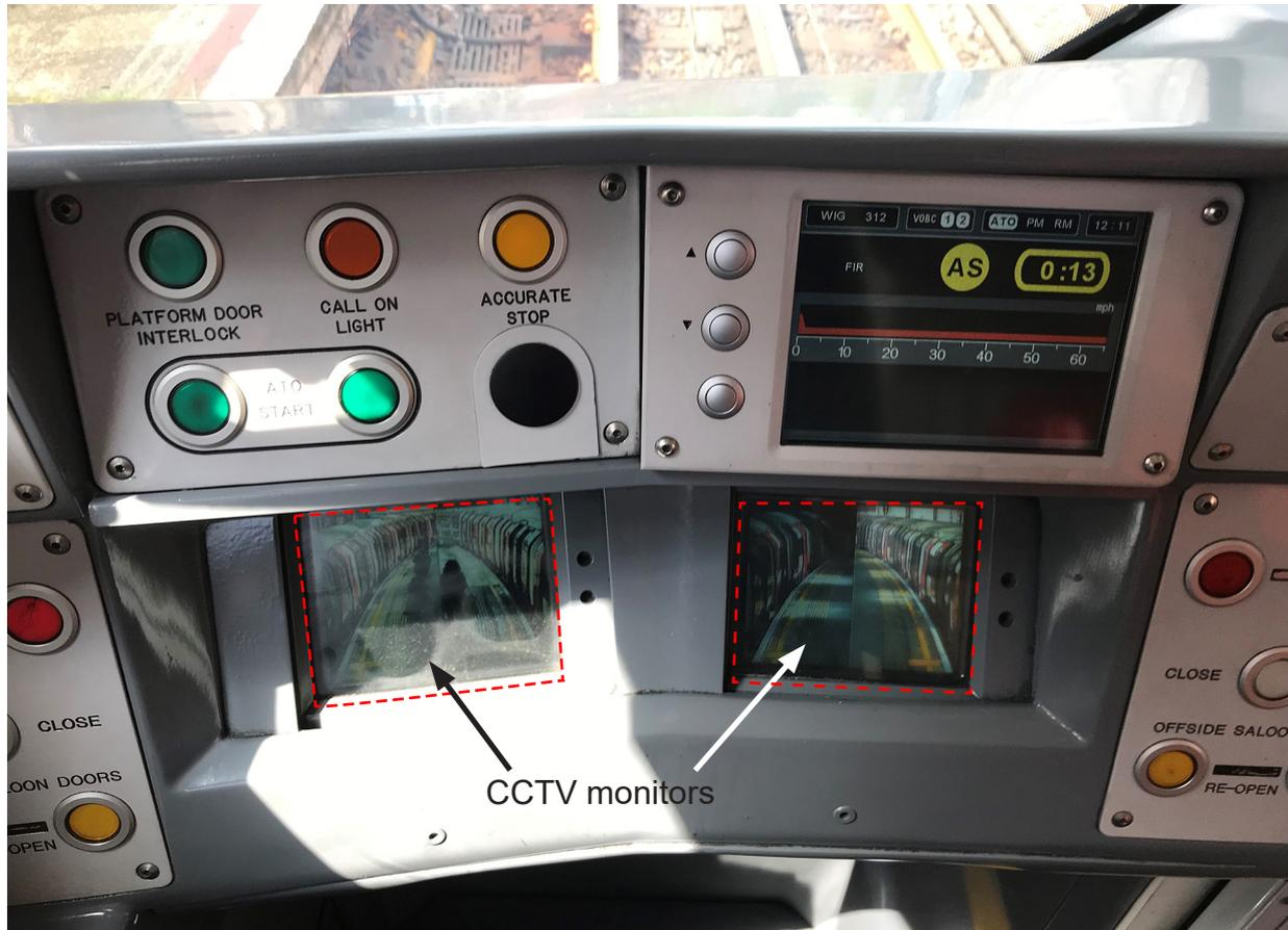
Figure 16: In-cab CCTV monitors showing longitudinal images of the side of a train
