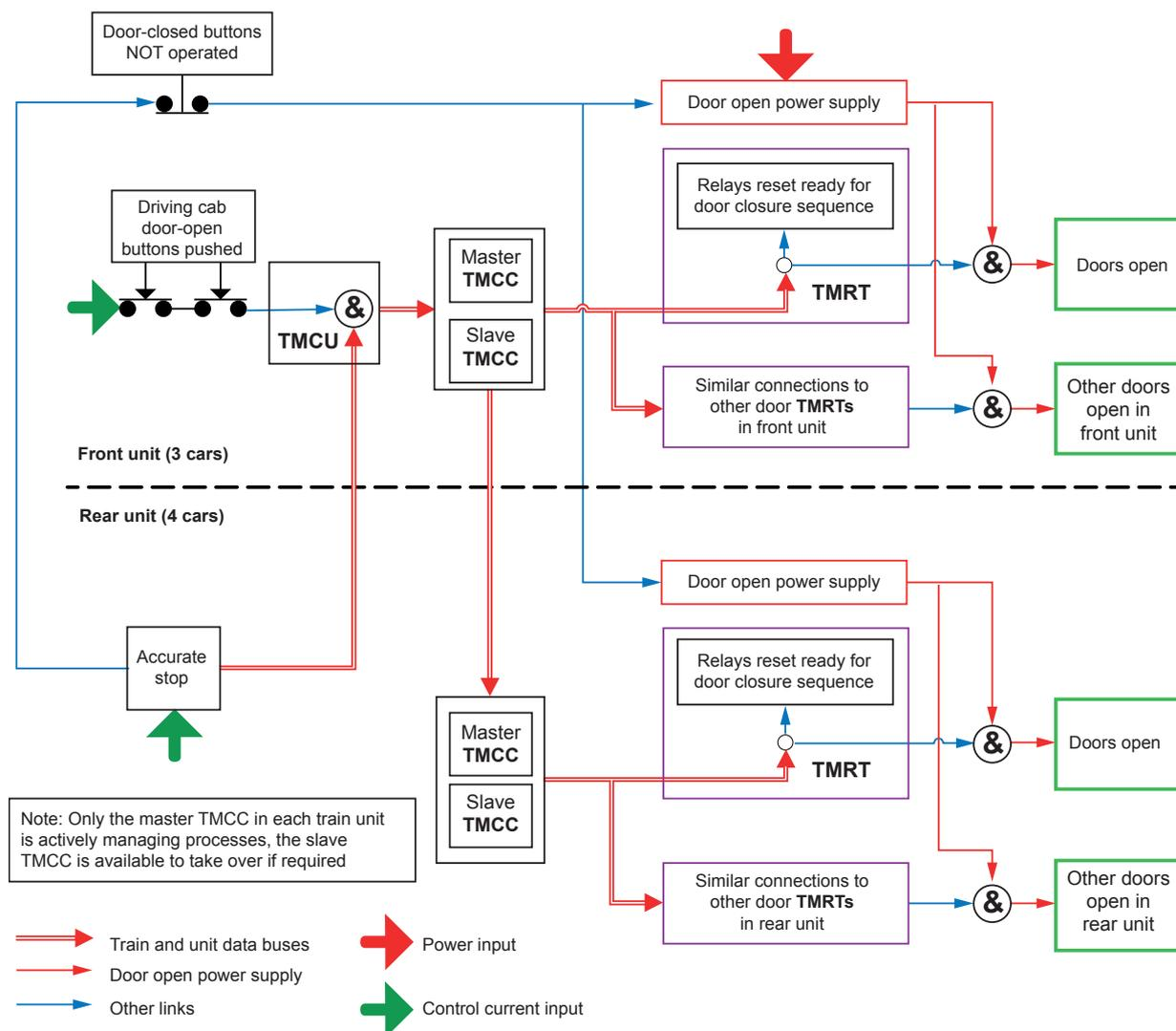
Figure C1: Door opening system, normal operation with train stopped accurately (simplified)
