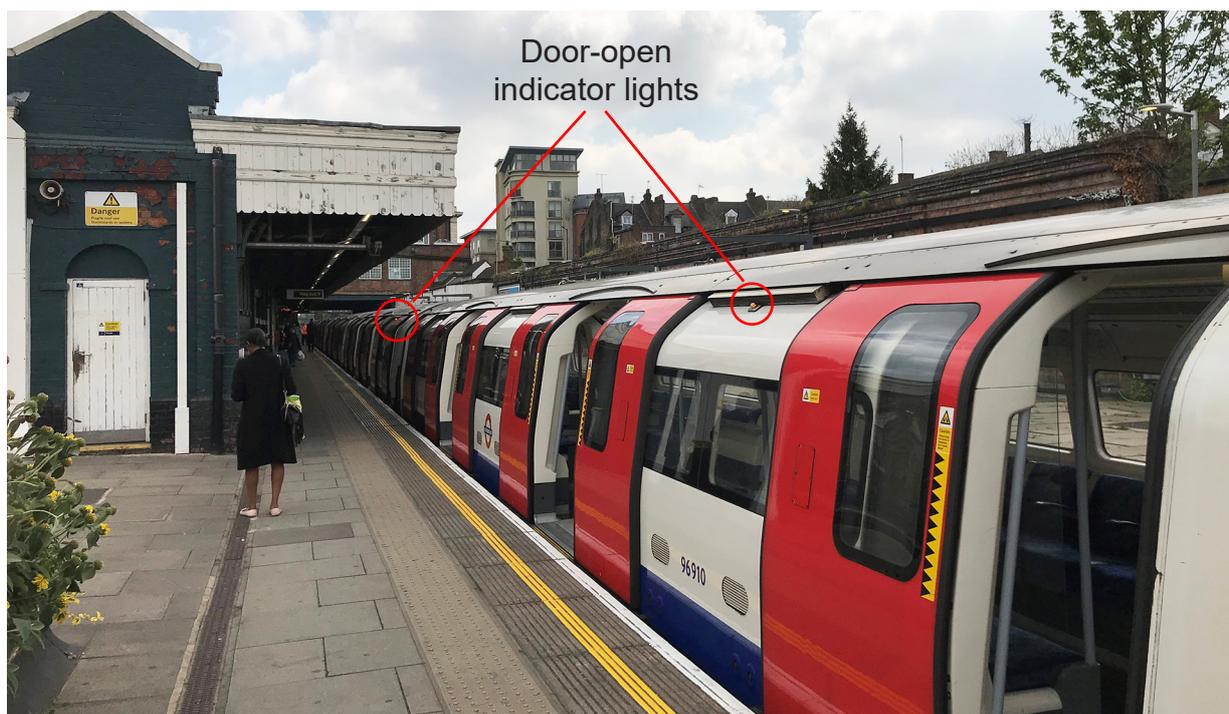
Figure 17: Door open indicator lights on outside of train
