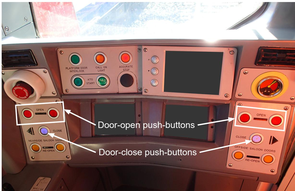
Figure 6: Train operator's passenger door-open and close buttons
