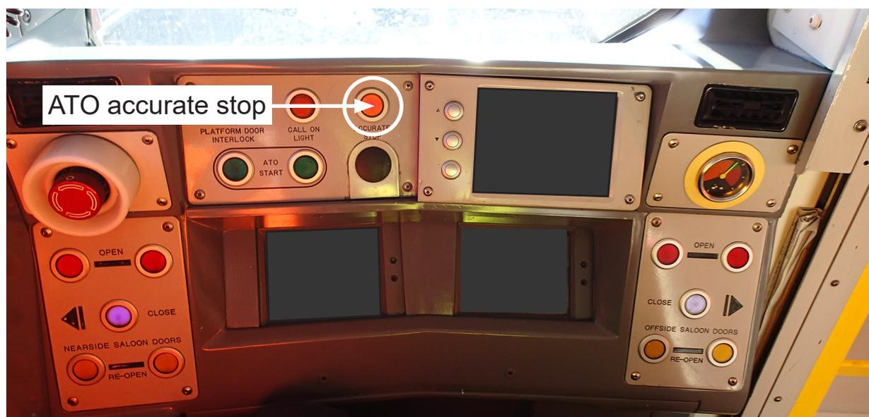
Figure 13: ATO accurate stop indicator
