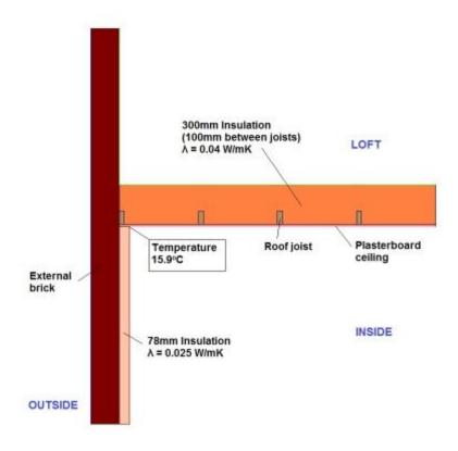
In the case of external wall insulation although the risk is lessened, it is not necessary when considering surface mould growth risk, to insulate past the height of the loft insulation level.
