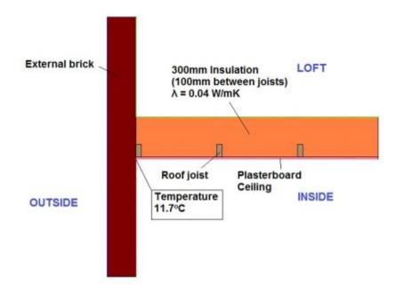
This risk can be mitigated by insulating the adjacent wall (either internally<sup>1</sup> or externally<sup>2</sup>).
