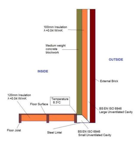
The lowest calculated internal surface temperature  $(T_{si})$  is 8.3°C. With an external temperature of 0°C, the resultant f<sub>Rsi</sub> is 0.42, which indicates a risk of mould growth.
