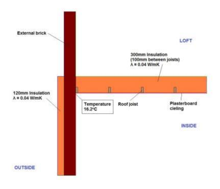
Two types of junctions have been identified where mould growth risk will be made worse by insulating the adjacent element - in these cases the addition of floor insulation increases the mould growth risk. There is another case where a balance needs to be reached between the requirement for thicker thermal insulation (to improve the building's energy efficiency) and thinner thermal insulation (to reduce or avoid moisture risk). These two are:
