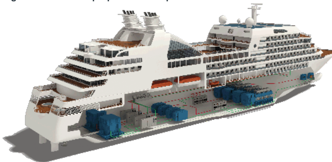
Figure 33 Electric propulsion example
