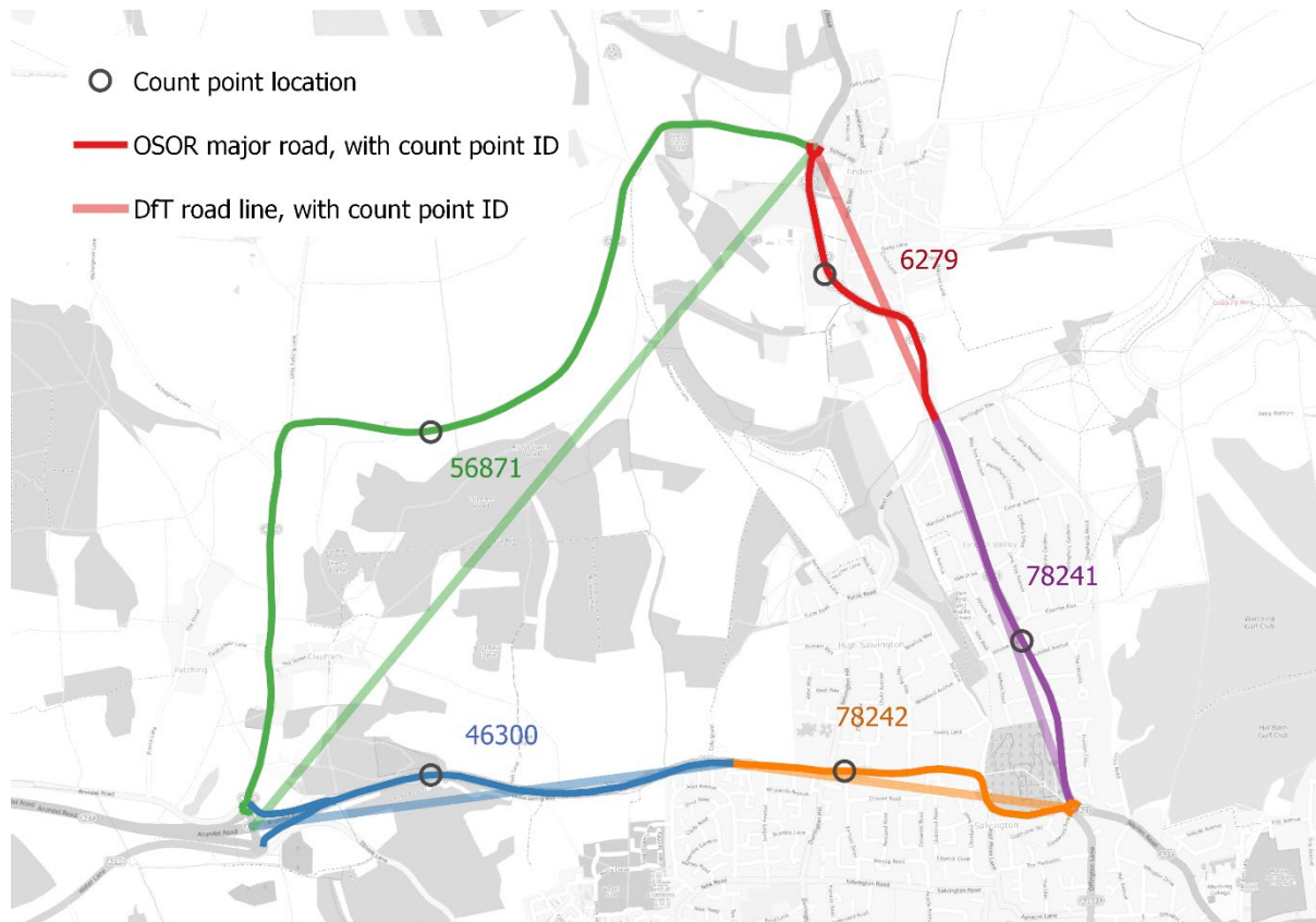
Figure 4: Traffic flows are assigned to the road network (Ordnance Survey Open Roads) by selecting OSOR sections that fall between the start and end points of traffic census count point coverage (DfT road line).
