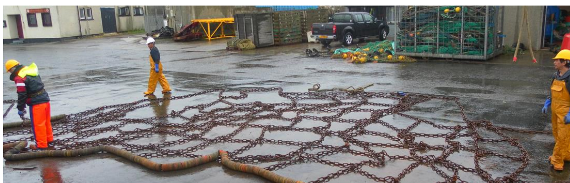
Figure 9.4: Chain mats for removal of clay berms
