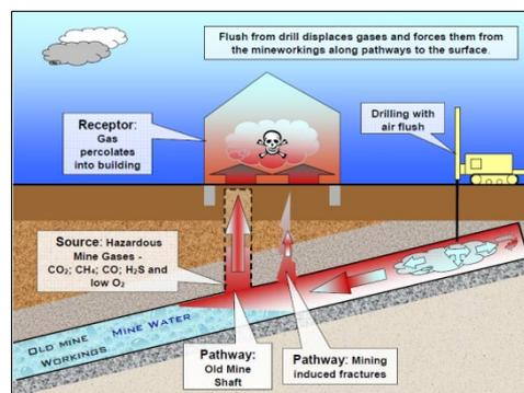
**Diagram 2** - shows how mine working investigations can cause hazards outside the site boundaries
