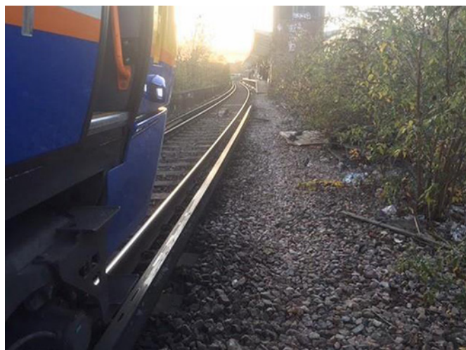
The steps used by passengers who were detrained from a failed train near Peckham Rye station (showing the position of the bottom step relative to the conductor rail).
