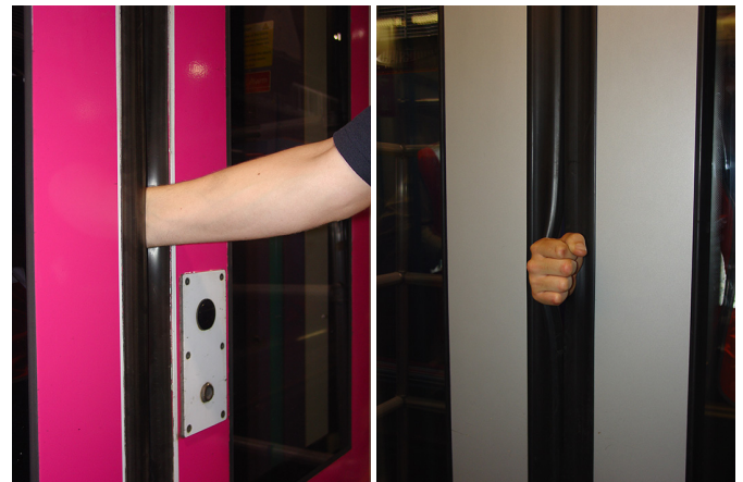
How a modern door detection system failed to detect the presence of a trapped hand (Newcastle Central in 2013 ( Report 19/2014 ), and again at Bushey in 2018)
