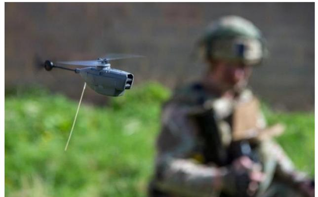
Pictured is a Royal Marine controlling a Black Hornet 2 Remotely Piloted Aircraft System
