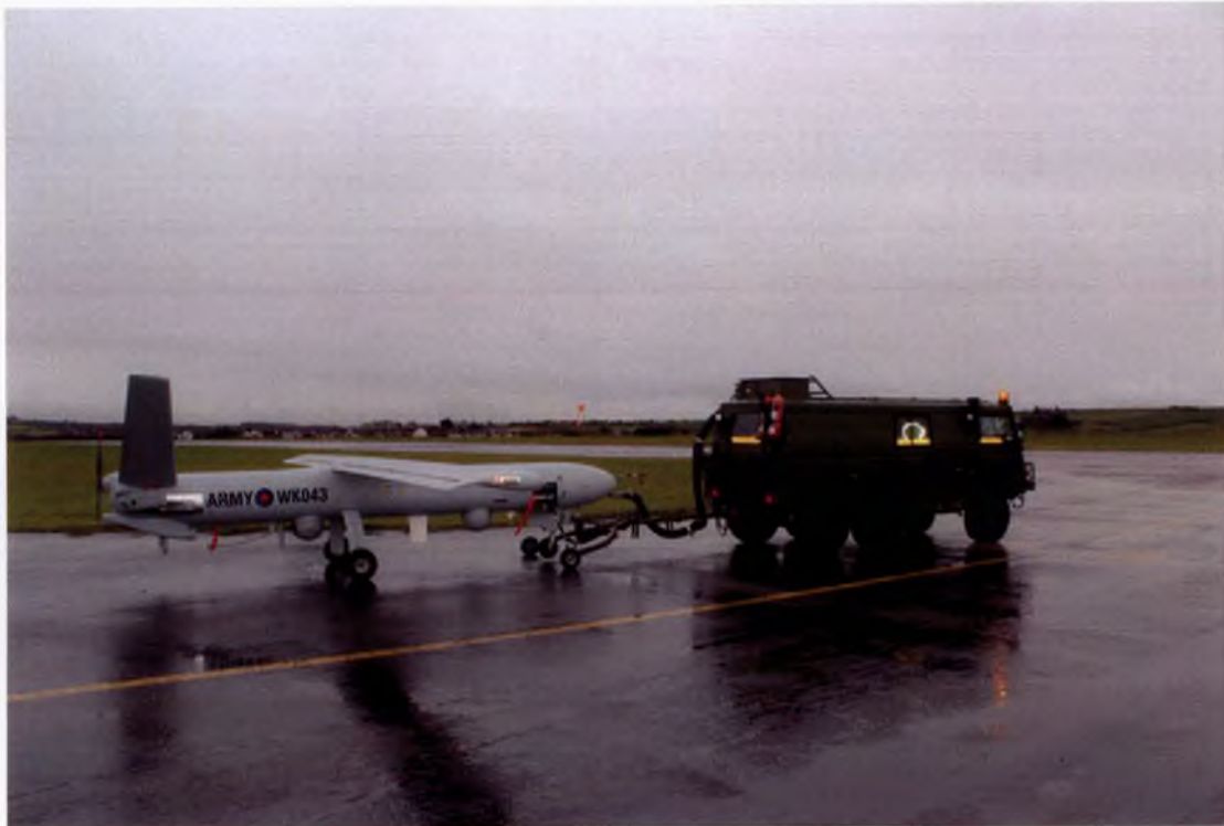
Figure 1.2.10 – A Pinzgauer vehicle equipped with a PATE towing WK to departure point
