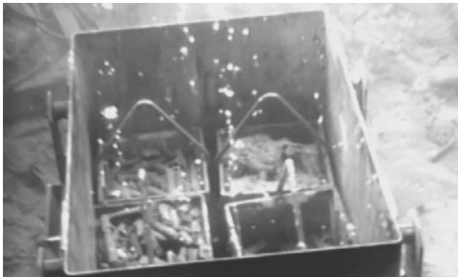
Photograph of the skip used in the trial during transport into the export cell. Bubbles of hydrogen gas can be seen emerging from the bins due to agitation during transport.
