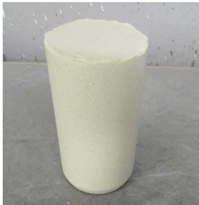
Geopolymer product with 70 vol % clinoptilolite waste loading.
