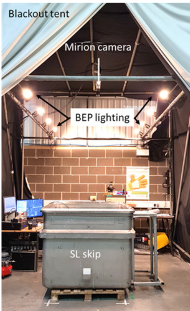
Photograph of the phase 2 test rig with BEP lighting using a Sellafield Ltd skip and a Mirion full resolution camera.
