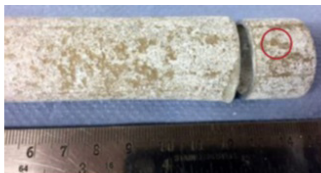
1050A grade aluminium sample corroded in \text{Mg}(\text{OH})_2 revealing two distinct corrosion regions (brown and white)
