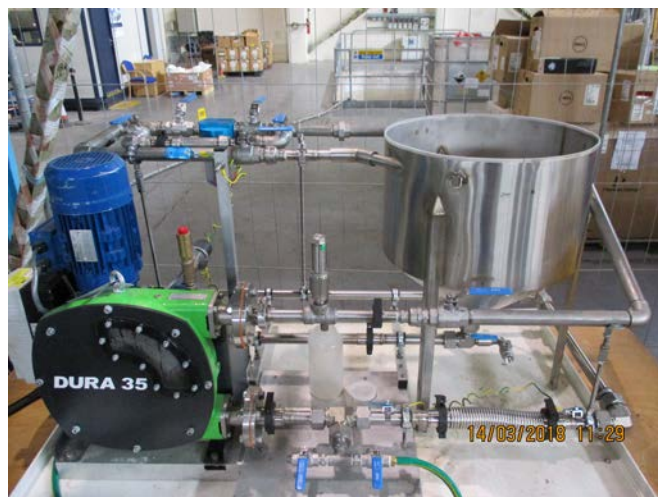
Image of the rig used to circulate and recover magnetic ion exchange material
