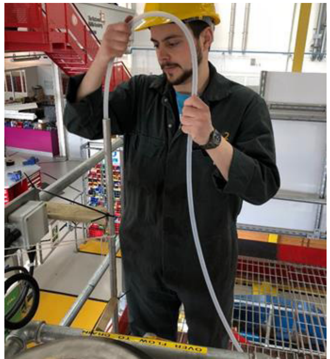
The picture shows the sheath material being deployed down the mock version of the 17m pneumericator line. Following deployment of the sheath, the camera is then deployed down the line inside the sheath.
