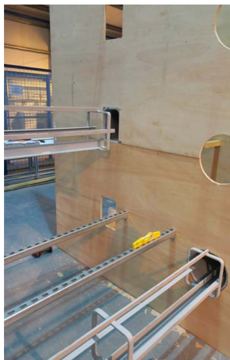
Completed North Store Test Rig: The completed rig replicates the physical constraints of the store in the dark environment
