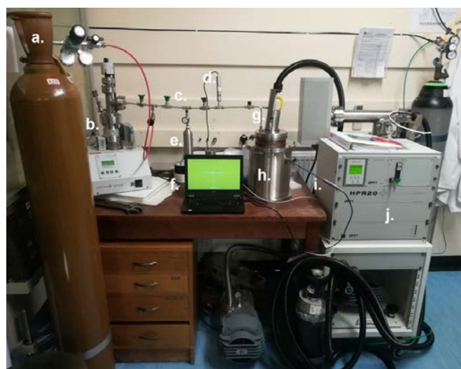
Gas control rig specifically designed for the project consisting of He cylinder, vacuum pump applying ultra-high vacuum, bellows and bonnet needle valves, high-speed pressure transducer, 300ml volume vessel, software controlling computer, mass spectrometer sample head, custom-designed cylindrical stainless-steel vessel sampling volume, temperature probe, mass spectrometer
