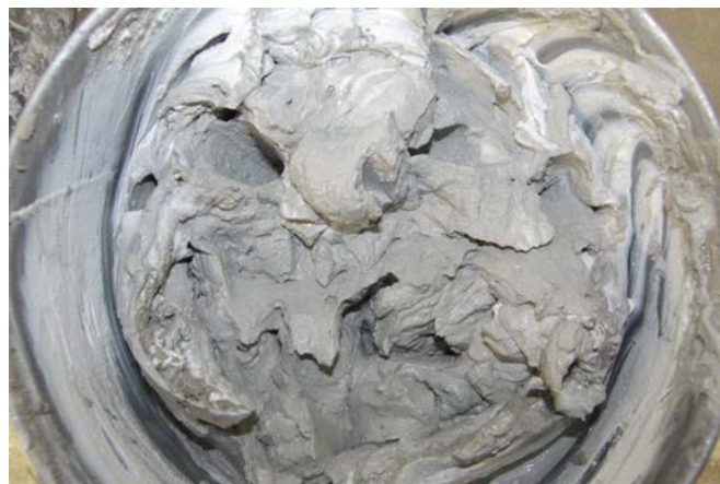
40 wt% CMS sludge at 60 vol % loading in (left) geopolymer and (right) 4.5:1 BFS/OPC @w/s 0.35. The difference in mixing viscosity can clearly be seen.
