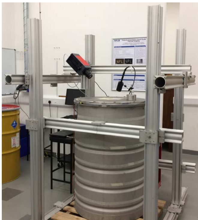
Phosphor thermometry experimental set up: This technique provides a robust method to remotely determine the temperature of a surface. A thin coating of thermographic phosphor is sprayed on the surface to be measured, this is excited with ultra violet light. The phosphorescence decay is then measured and the decay time determined, this is directly related to temperature through calibration
