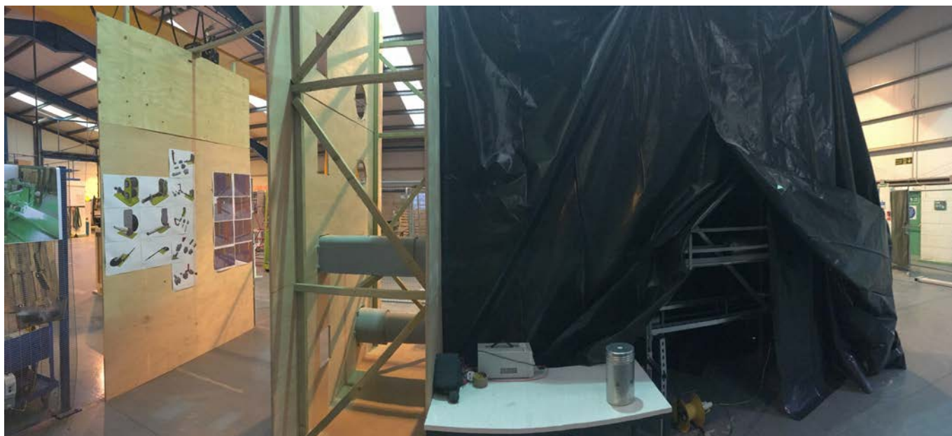
Completed North Store Test Rig: The completed rig replicates the physical constraints of the store in the dark environment
