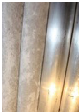
Left: Aluminium samples (1050A grade), corroded in saturated \text{Mg}(\text{OH})_2 for 9 months. Right: clean aluminium samples
