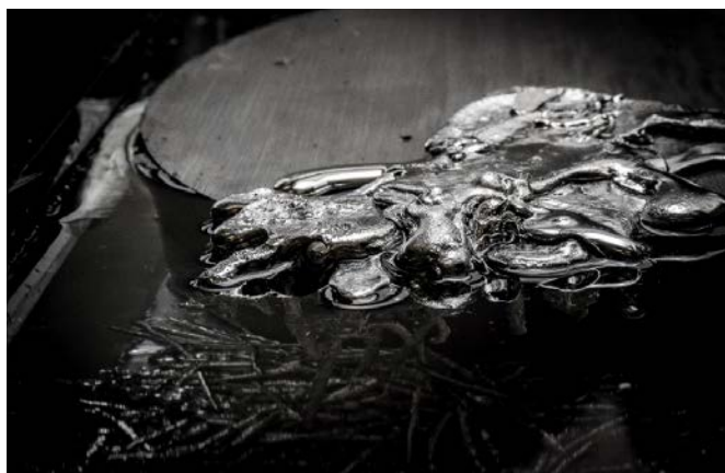
The Bismuth Plug, developed by Rawwater Engineering for sealing oil and gas wells during decommissioning, is a metal alloy with a composition that can be tailored to expand when it solidifies, potentially a novel system for containment of radioactive surfaces ( www.rawwater.com )
