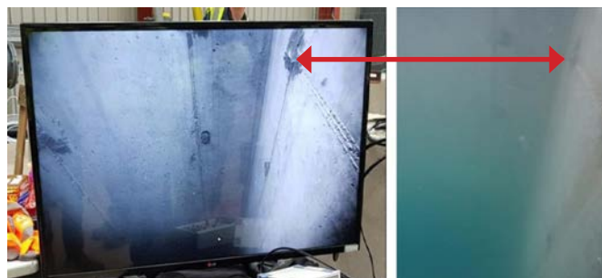
The image on the left is the output from the low light camera, compared with the image on the right, taken with a normal camera
