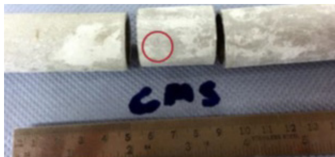
1050A grade aluminium sample corroded in CMS, visual inspection indicated two distinct corrosion regions: grey/brown and white
