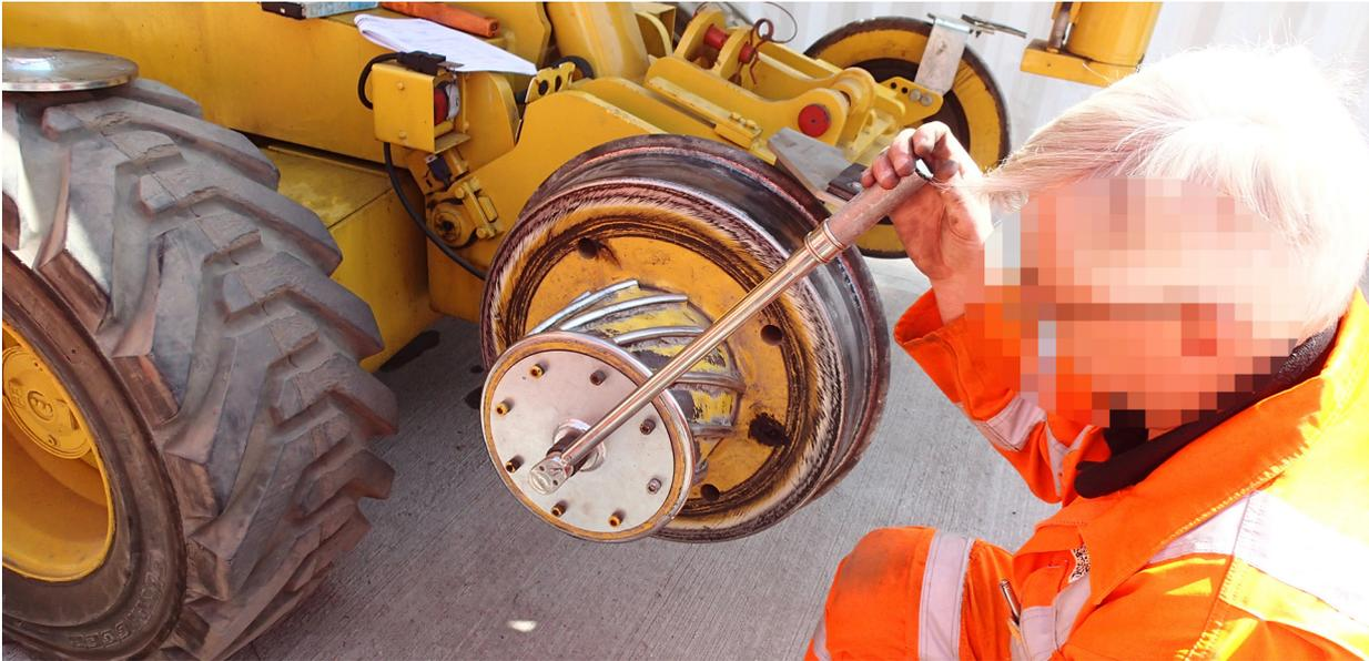
Figure 15: Torque testing of DRWB system
