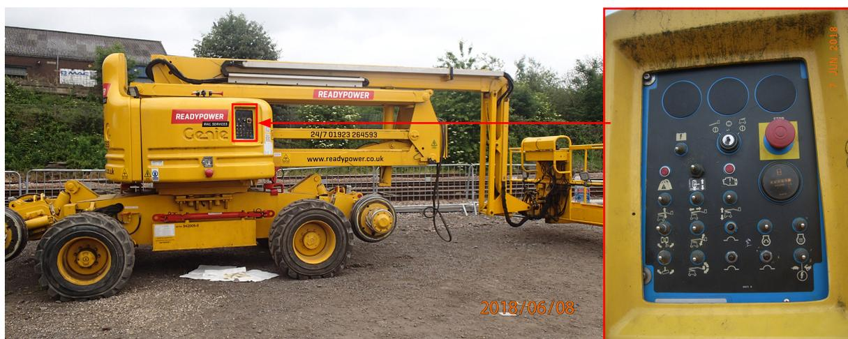
Figure 8: Control panel attached to the body of the MEWP
