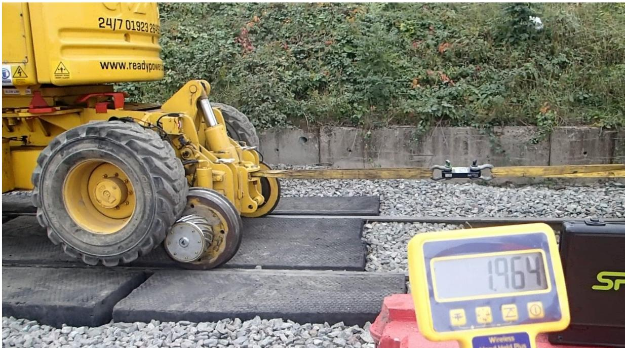
Figure 16: Pull-test when road wheels acting only (DRWB callipers removed)
