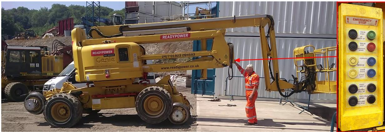
Figure 21: Operator pressing the rail axle deployment button at bottom of pendant
