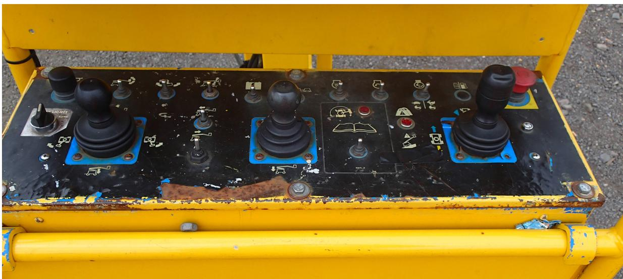
Figure 7: Control panel in the operator's basket
