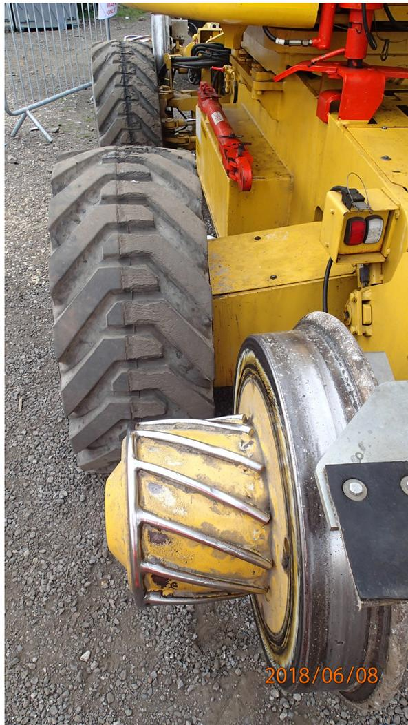
Figure 4: Hubs at the end of the rail axles
