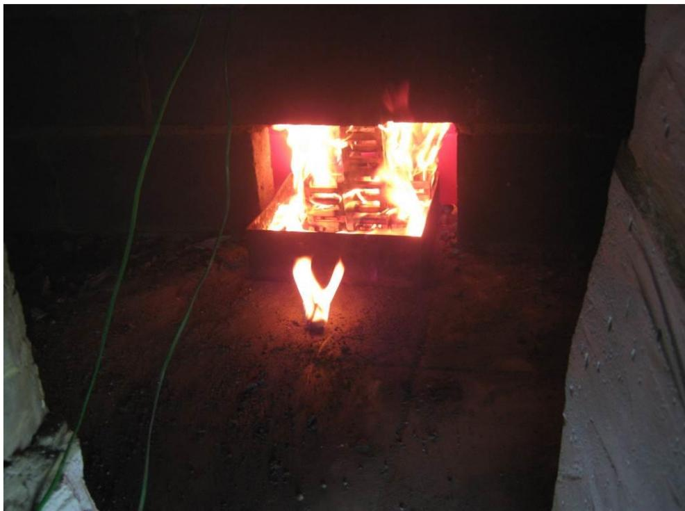
**Figure 26 - Ignition source and ventilation opening at low level**
