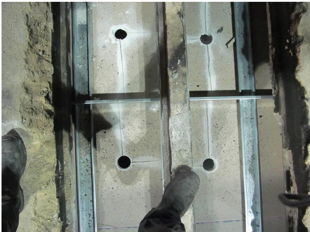
**Figure 18 - Holes drilled through plasterboard in centre of fire compartment (The finished roof with the location of the intermediate spandrel panel indicated by yellow paint is shown in Figure 19)**
