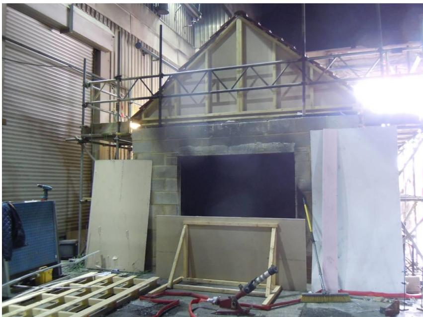
**Figure 15 - (Northern) Gable end showing plasterboard to internal face of spandrel panel**
