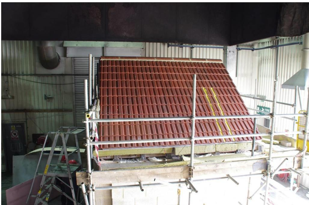
**Figure 19 - Completed roof structure with spandrel panel location indicated by yellow paint**
