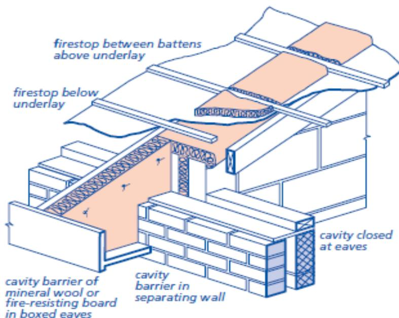
**Figure 2 - Detail of fire stopping at wall/floor junction (From NHBC Design standard Part 7 Roofs Chapter 7.2 Pitched roofs<sup>8</sup>)**
