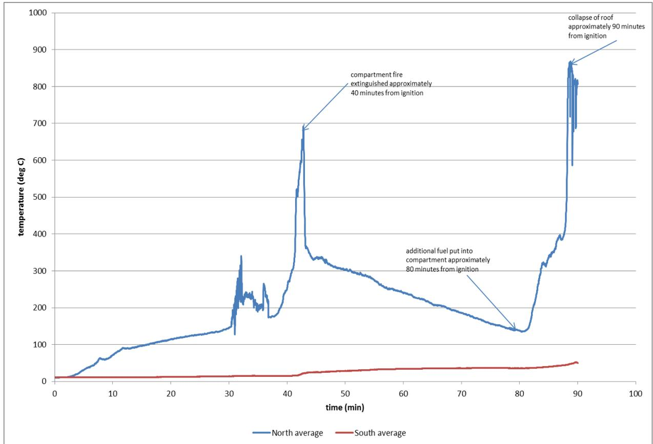
**Figure 21 - Average temperatures in roof void either side of compartment wall**
