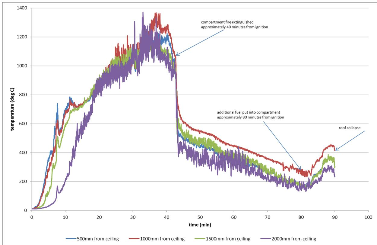
**Figure 20 - Compartment temperatures (North West corner)**
