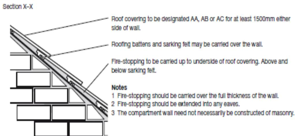
**Figure 1 - Section showing typical detailing for fire stopping between compartment wall and roof covering (from Diagram 30 of Approved Document B)**
