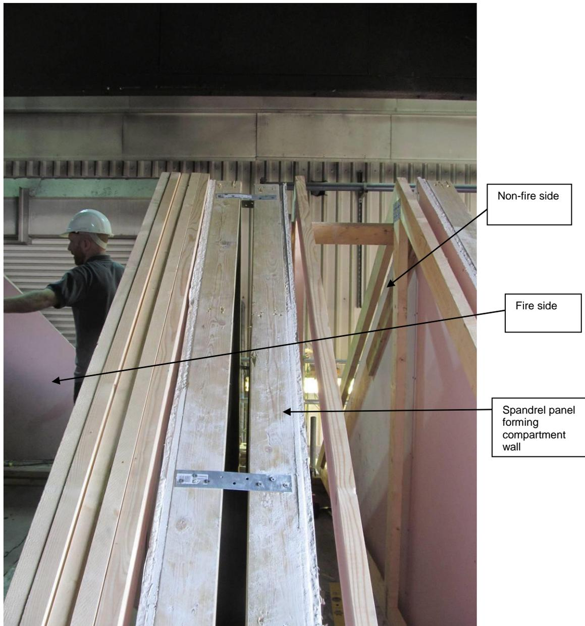
**Figure 16 - Intermediate spandrel panel showing double layer plasterboard protection**
