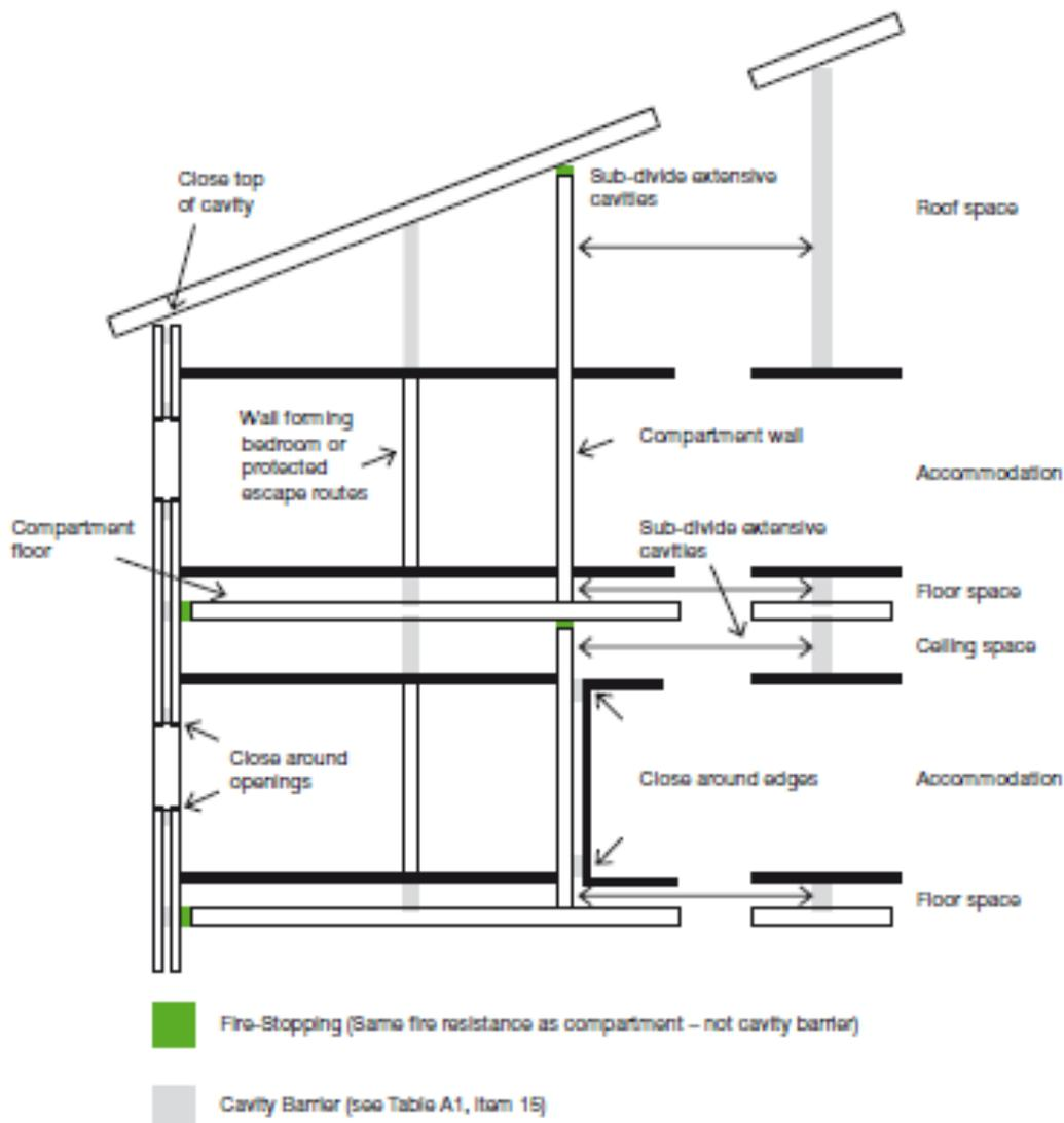
Figure 23 - Provisions for cavity barriers (Diagram 33 of Approved Document B<sup>1</sup>)
