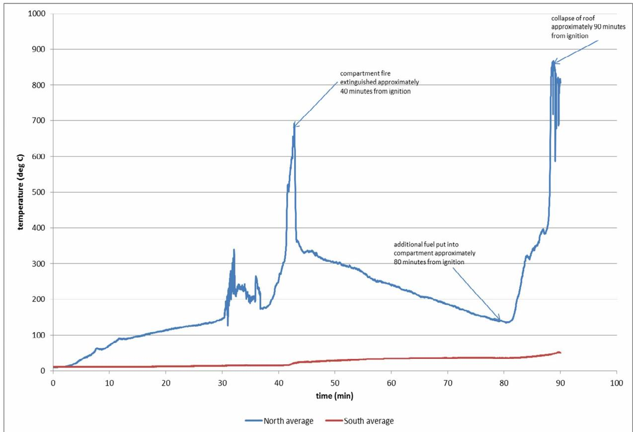
**Figure 9 - Average temperatures in roof void either side of compartment wall**
