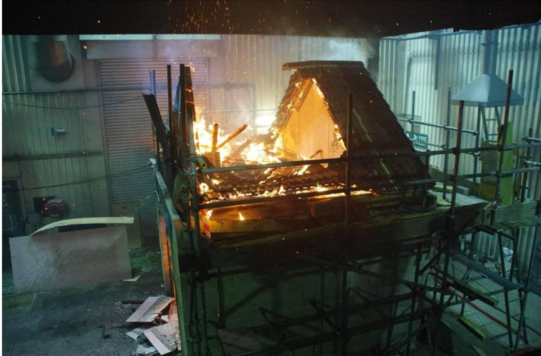
**Figure 10 - Collapse of roof structure with compartmentation intact**
