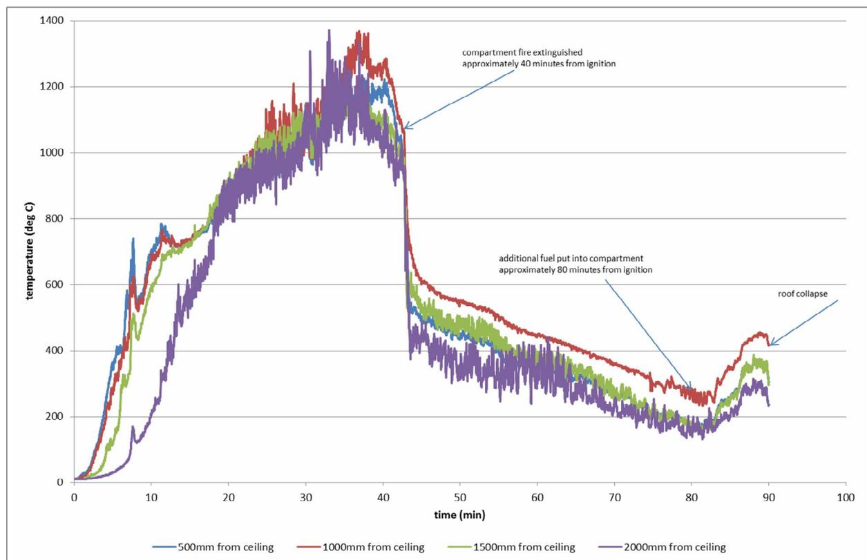
**Figure 8 - Compartment temperatures (North West corner)**
