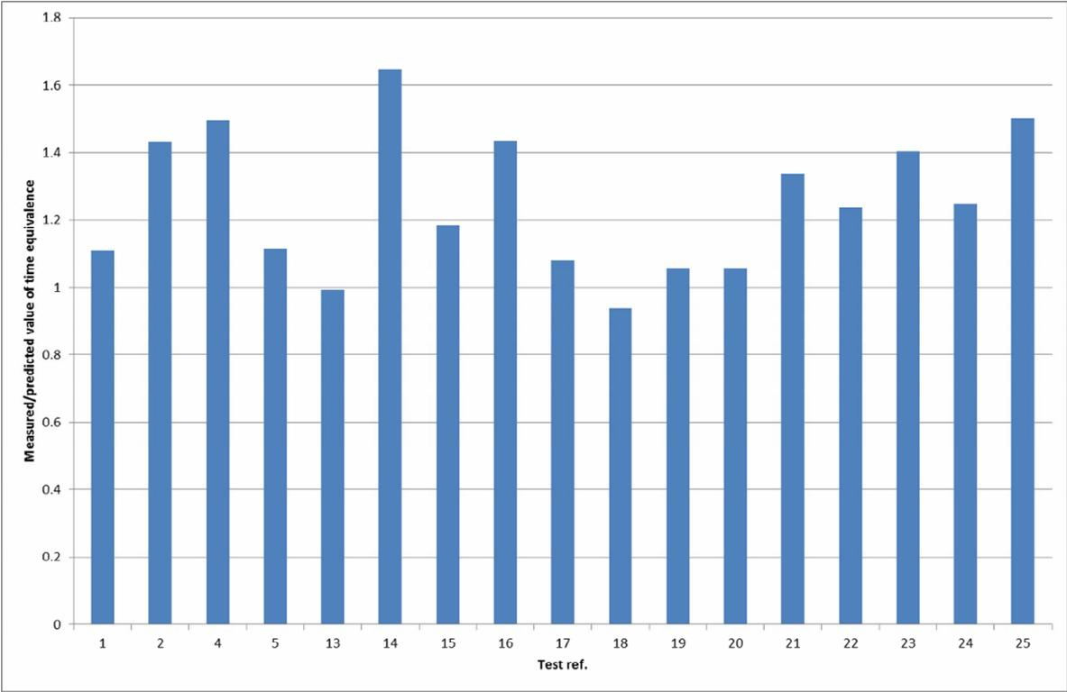
**Figure 7 - Comparison between measured and predicted values of time equivalence for a range of large-scale fire tests**
