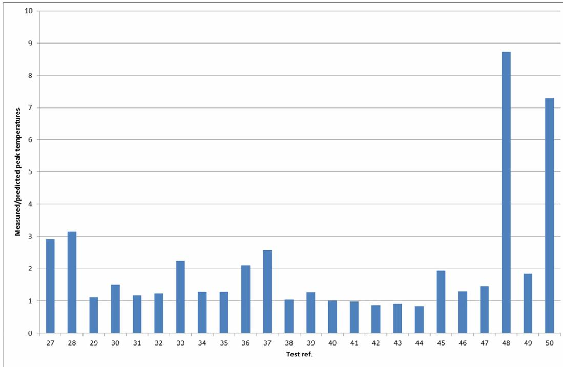
**Figure 3 - Comparison between measured and predicted peak temperatures for BISF tests**
