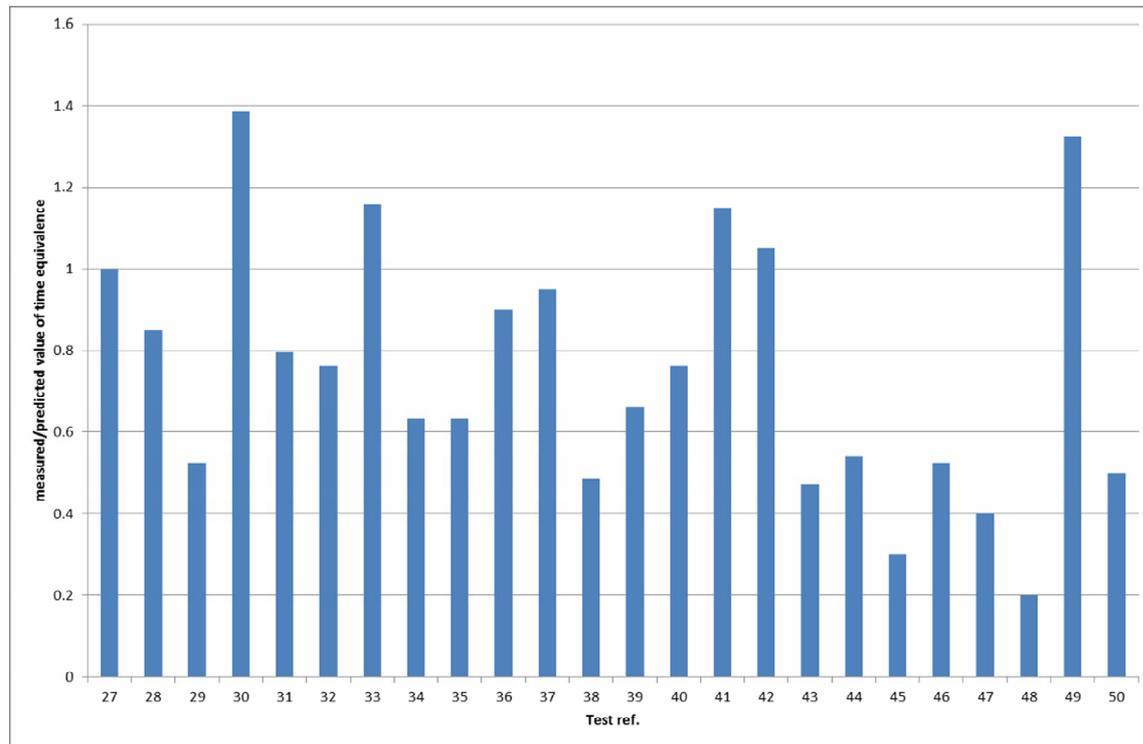
**Figure 8 - Comparison between measured and predicted values of time equivalence for BISF tests**
