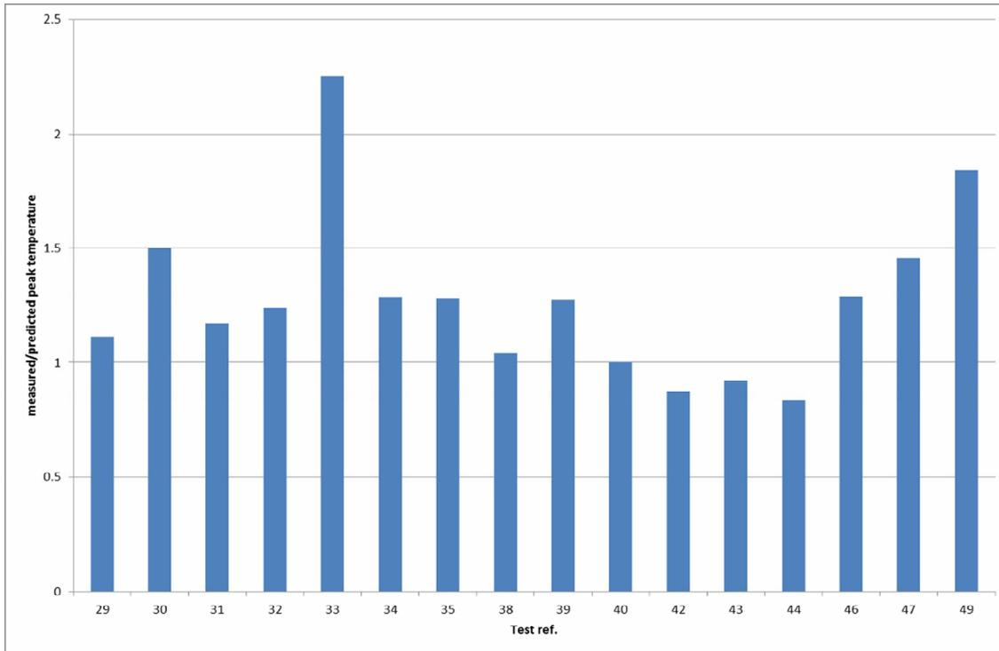
**Figure 4 - Comparison between measured and predicted peak temperatures for BISF tests with low fire load values removed**
