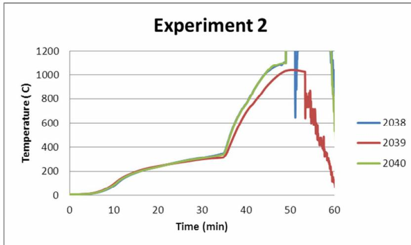
**Figure 20 - Temperatures of indicative column element for Experiment 2**
