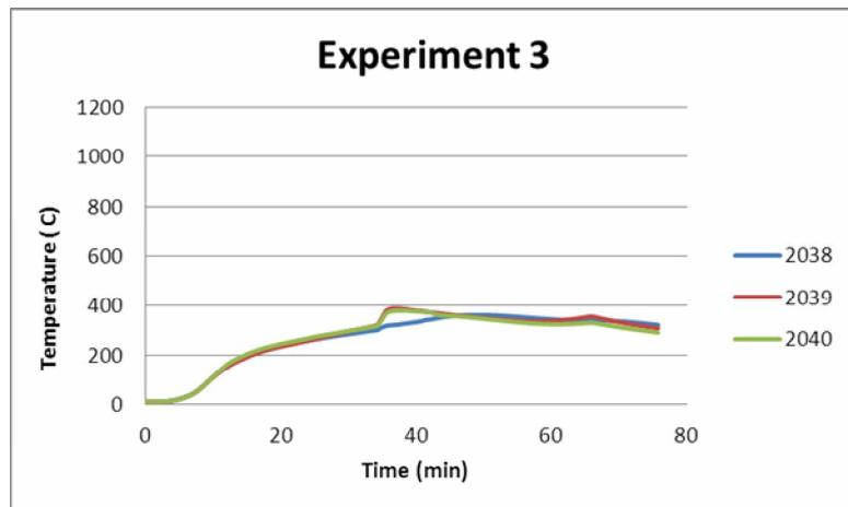
**Figure 24 – Temperatures of indicative column element for Experiment 3**
