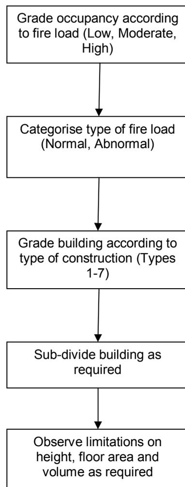
**Figure 1 - Methodology underpinning Fire Grading of Buildings**
