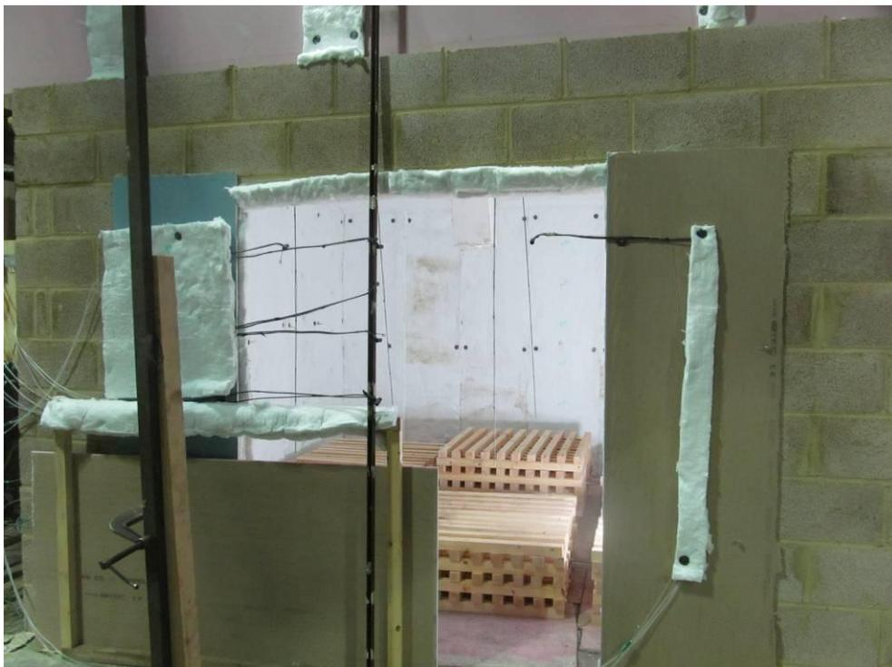
**Figure 9 - View of the fire compartment looking in from front ventilation opening**
