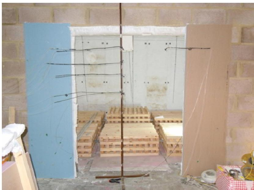
**Figure 11 - View of cribs inside rig prior to Experiment 1**
