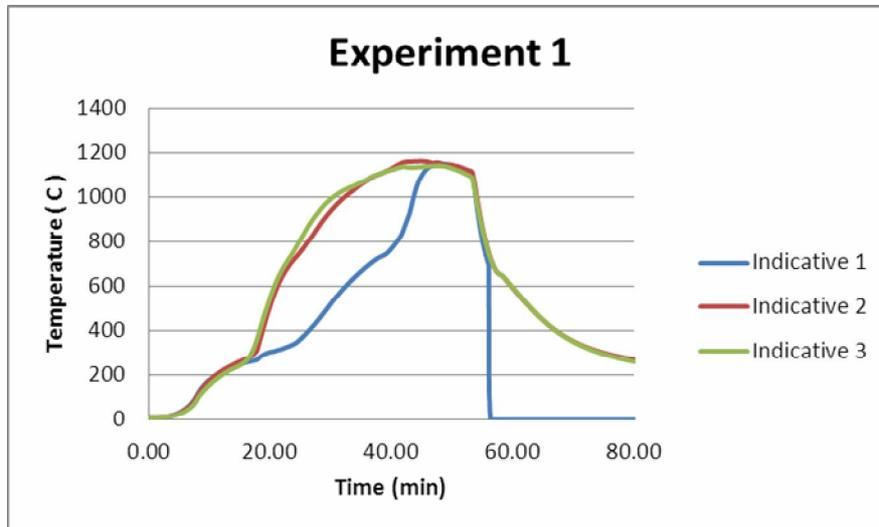
**Figure 15 - Indicative column element temperatures for Experiment 1**
