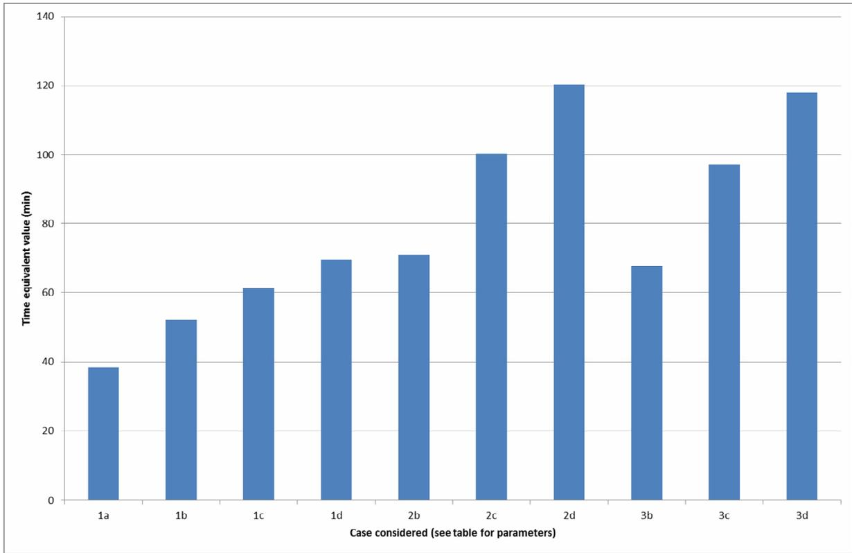
**Figure 27 - Effect of variation in fire load density and ventilation conditions**
