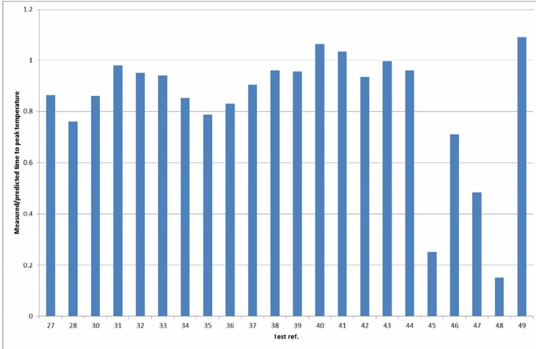
**Figure 6 - Comparison between measured and predicted time to peak temperature for BISF fire tests**
