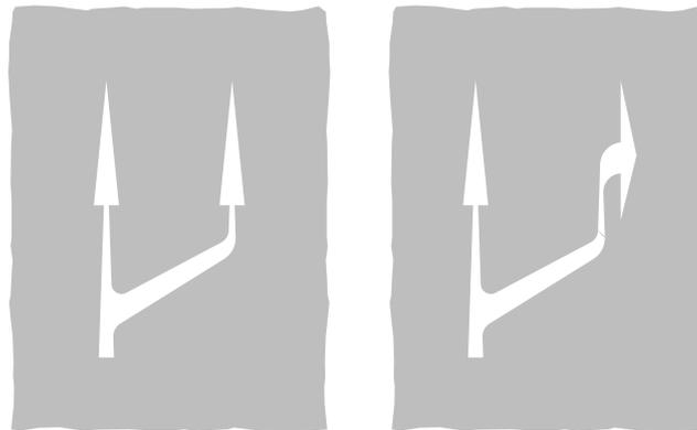
**Figure 9-7** Diagram 1050.1 (S9-6-13) Indication of traffic movements at end of off-side bus lane or intermediate junction (Alternative types)
