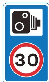
**Figure 8-17** Diagram 880 (S11-2-64) Speed camera ahead on a lit road and reminder of 30 mph speed limit
