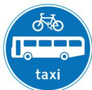
**Figure 9-22** Diagram 953 (S3-2-33) Route for use by buses, pedal cycles and taxis only (Alternative types)
