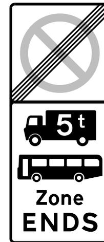
**Figure 14-5** Diagram 666 (S7-2-2) End of a controlled parking zone applying to goods vehicles, buses or both
