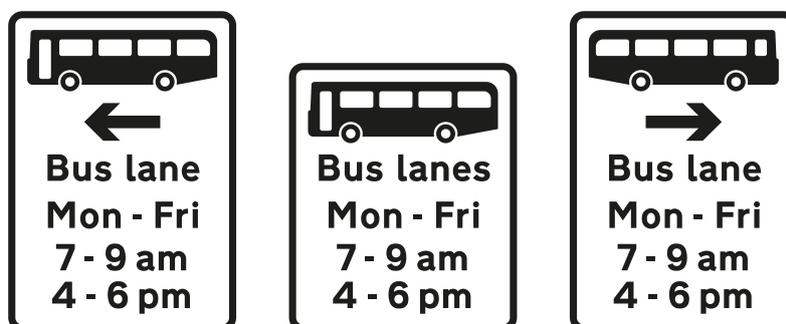
**Figure 9-9** Diagram 962 (variant) (S11-2-34) Bus lane on road at junction ahead with indication of times of operation (Alternative types)
