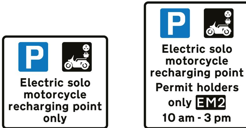
**Figure 13-45** Examples of upright signs prescribed by S4-4 and 5 indicating a parking place reserved for the recharging of electric solo motor cycles
