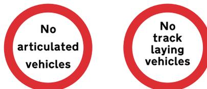
**Figure 5-15** Diagram 622.4 (S3-2-15) Articulated or track laying vehicles prohibited (Alternative types)
