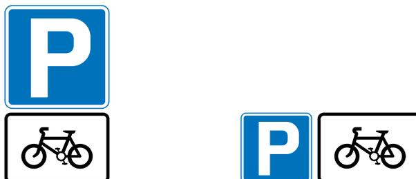
**Figure 11-31** Diagrams 968 and 968.1 (S11-2-47) Parking place for pedal cycles
