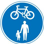
**Figure 11-18** Diagram 956 (S3-2-29) Route for use by pedal cycles and pedestrians only
