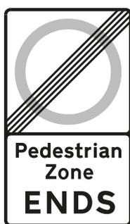
**Figure 6-4** Diagram 618.4A (S8-2-3) End of restrictions associated with a pedestrian zone
