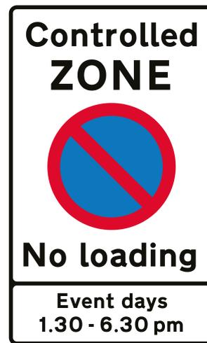
**Figure 14-3** Example of a lower panel on a type (a) CPZ entry sign indicating “Event days”
