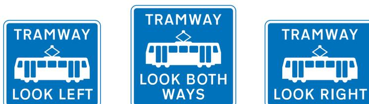
**Figure 10-13** Diagram 963.3 (S11-2-43) Direction in which pedestrians should look for approaching tramcars when crossing a tramway (Alternative types)
