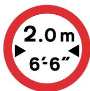
**Figure 5-26** Diagram 629A (S3-2-26) Width restriction in metric and imperial units
