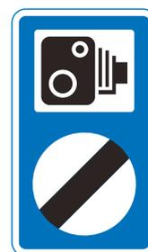
**Figure 8-18** Diagram 880.1 (S11-2-65) Speed camera ahead on an unlit road and reminder that a national speed limit applies
