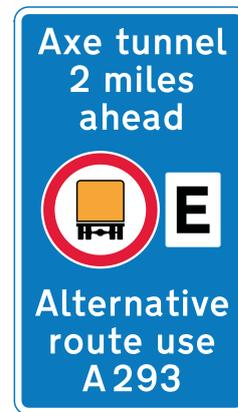
**Figure 5-21** Diagram 818.4 (permitted variant) (S12-28-22) Tunnel restriction ahead for vehicles carrying dangerous goods with indication of alternative route
