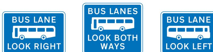
**Figure 9-19** Diagram 963 (S11-2-40) Direction in which pedestrians should look for approaching traffic when crossing a bus lane (Alternative types)
