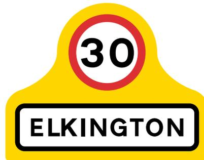
**Figure 8-21** Example of a speed limit sign co-located with a boundary sign
