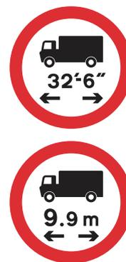
**Figure 5-27** Diagram 629.1 (S3-2-25) Length restriction in imperial and metric units
