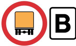
**Figure 5-20** Diagram 622.10 (S9-4-3) Vehicles carrying dangerous goods within the tunnel restriction code indicated by the sign prohibited
