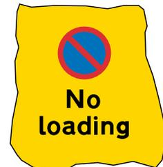
**Figure 13-88** Diagram 640.1 (S13-6-22) Waiting, loading and unloading prohibited at a parking place where parking is temporarily suspended
