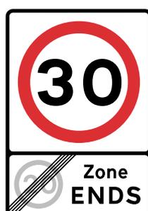
**Figure 8-10** Diagram 675A (S10-2-6) End of 20 mph speed limit zone with indication of maximum speed limit in mph
