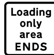
**Figure 13-81** Diagram 664.2 (S7-2-4) End of loading only area
