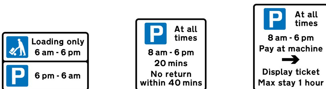
Figure 15-3 Examples of upright signs indicating loading and parking bays where controls do not apply throughout the operational period of the restricted parking zone
