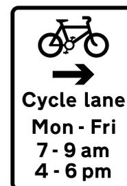
**Figure 11-5** Diagram 962.1 (S11-2-35) Cycle lane on road at junction ahead (Alternative types)
