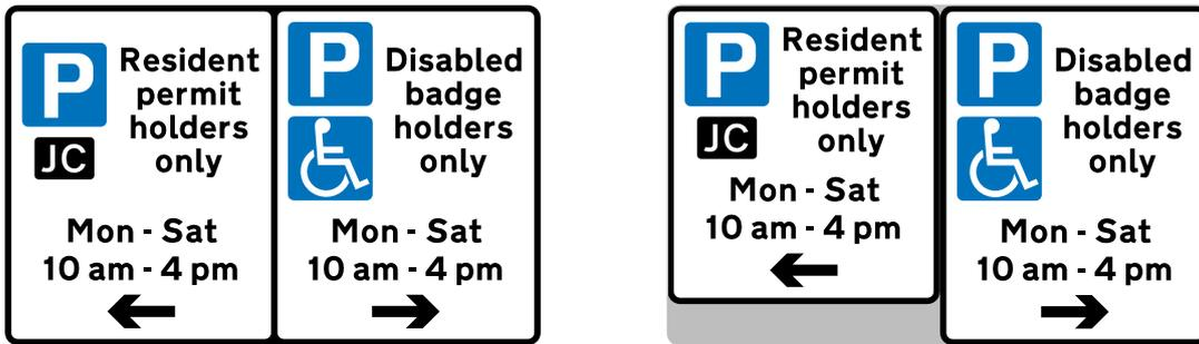
Figure 13-62 Signing arrangement for different parking bays side by side (Alternative types)
