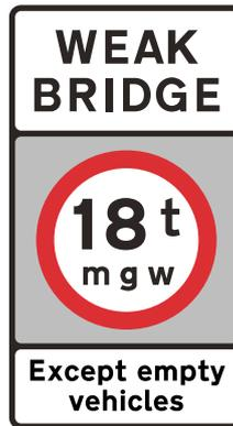
**Figure 5-25** Diagram 626.2A (S9-4-2) Maximum weight of vehicle on bridge with an exception for empty vehicles
