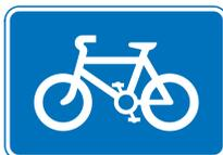
**Figure 11-7** Diagram 967 (S11-2-44) Route recommended for pedal cycles on the main carriageway of a road
