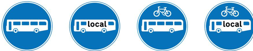
**Figure 9-16** Diagram 953 (variant) (S3-2-33) Route for use only by buses and, where indicated, pedal cycles (Alternative types)
