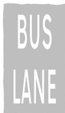
**Figure 9-4** Diagram 1048 (S9-6-14) Traffic lane reserved for buses and other vehicles as indicated on the sign to diagram 959B
