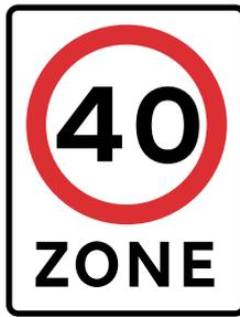
**Figure 8-6** Diagram 676 (S10-2-8) Entrance to a zone where a maximum speed limit of 40 mph is in force
