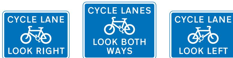
**Figure 11-16** Diagram 963.1 (S11-2-41) Direction in which pedestrians should look for approaching pedal cycles when crossing a cycle lane (Alternative types)
