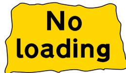
**Figure 13-87** Diagram 636.1 (S13-6-20) Temporary prohibition of loading and unloading
