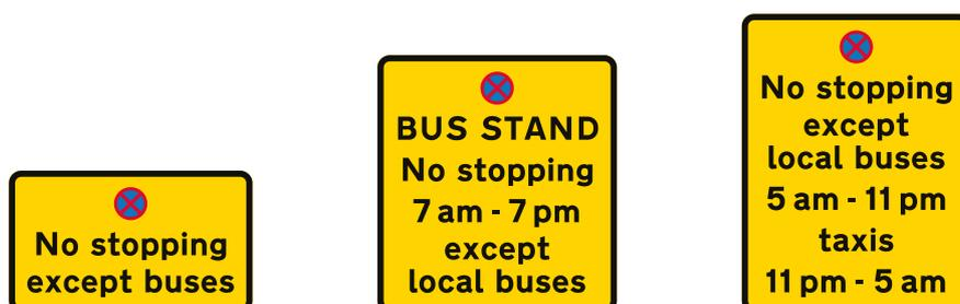
**Figure 13-72** Examples of upright signs indicating places where only buses may stop during the period indicated, for the purpose of picking up and setting down passengers and where a bus stop is used overnight as a "no stopping" taxi rank
