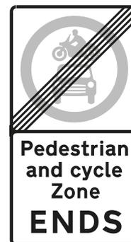
**Figure 6-5** Diagram 618.4B (S8-2-4) End of restrictions associated with a pedestrian and cycle zone
