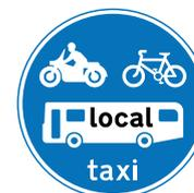
**Figure 9-24** Diagram 953B (S3-2-35) Route for use by buses, pedal cycles, solo motor cycles and taxis only (Alternative types)
