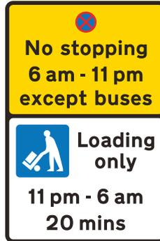
**Figure 13-73** Signing arrangement for a bus stop during the daytime and a loading bay overnight
