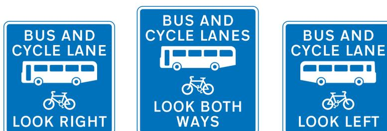
**Figure 9-20** Diagram 963.2 (S11-2-42) Direction in which pedestrians should look for approaching traffic when crossing a contraflow bus and cycle lane (Alternative types)
