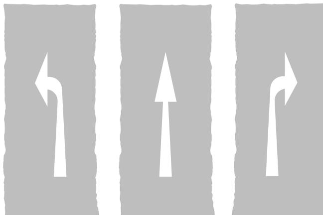
**Figure 11-30** Diagram 1059 (S11-4-32) Directions in which pedal cycles should travel along a cycle lane, track or route (Alternative types)
