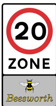
**Figure 8-9** Diagram 674 (S10-2-5) Entrance to a zone where a maximum speed limit of 20 mph is in force
