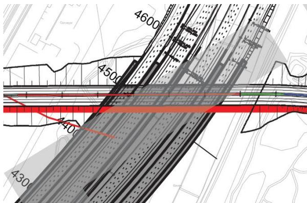
Once the river diversion & earthworks realignment is complete south of the old A4, Bath Road, then this road can be shut as access from it is no longer required. The earthworks realignment in this section can then progress and will marry up to the earthworks realignment in the previously demolished SSE pylons & Longford
