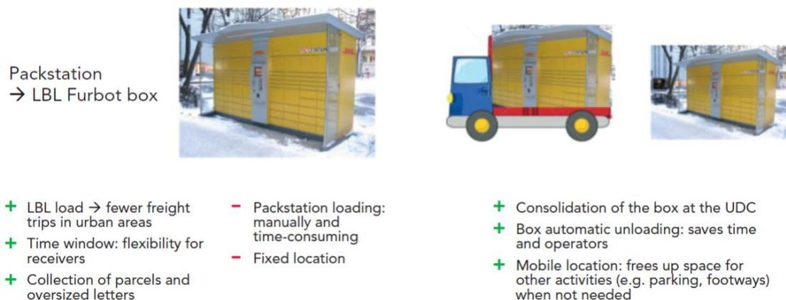
**Figure 8: FURBOT and the mobile Packstation concept<sup>24</sup>**
