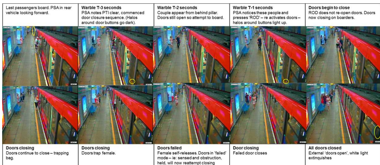
Figure 2: CCTV of door entrapment incident at Cutty Sark during 3-second door warning sound trial
