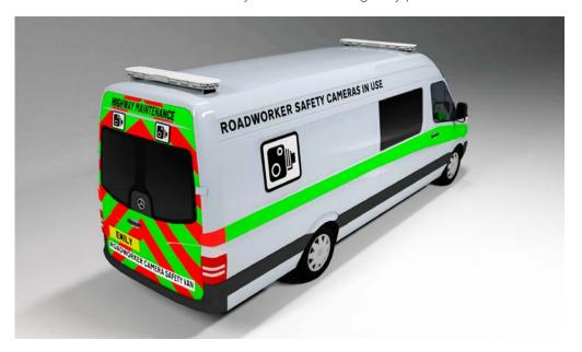
with livery similar to that used by the Safety Camera Partnerships. These vehicles are welfare vans that have been modified by the use of magnetic stickers. Trials taken place have shown the use of such vehicles have significantly reduced vehicle incursions and also a noticeable increase in traffic compliance with the road works speed limit
