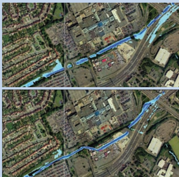
Top: Flood Risk Before – baseline Bottom: Flood Risk After – river diversion included Images courtesy of Scott Wilson and the Brent Cross Cricklewood Development Partners
