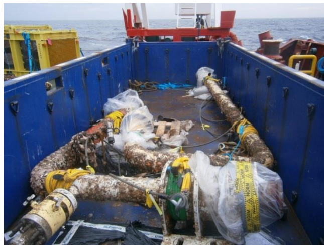
Figure 9.4.1: Pipe spools stored inside container
