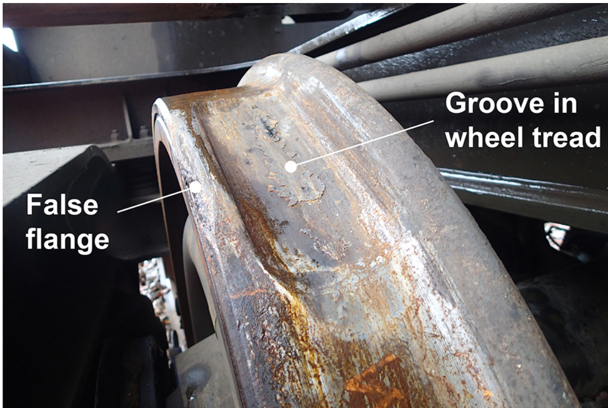
The large flat on the leading left-hand wheel of the 4 th bogie and its associated false flange
