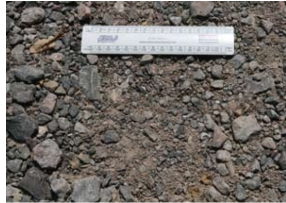
Impermeable hardcore or Type 1
