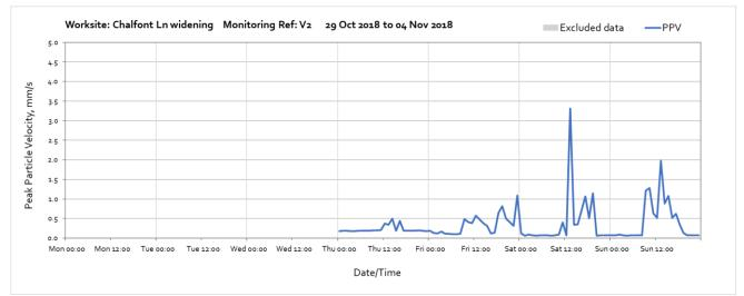
Note – Data until 11:00 on Wednesday 7<sup>th</sup> were due to vibration generated by houshold events occurring in proximity to the vibration monitor and not related to HS2 works.
