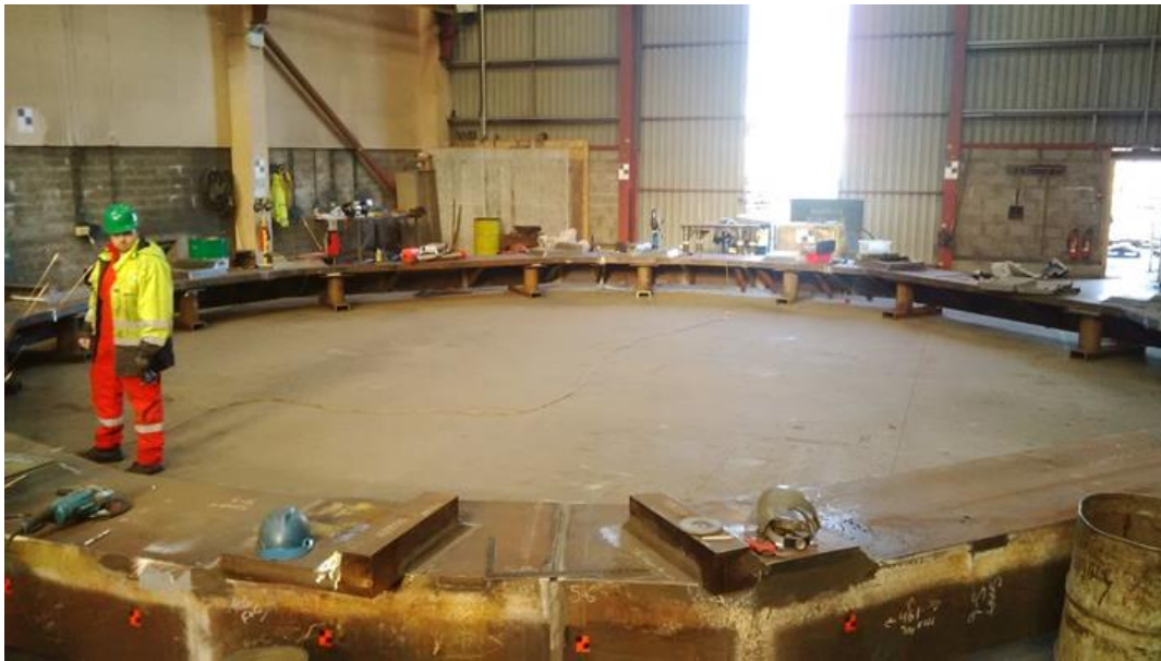
Figure 8. Shear Restraint being Assembled Dry Onshore.
