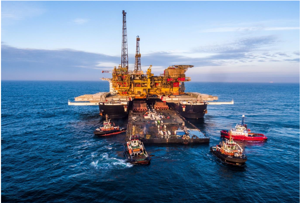
Figure 25. Inserting the Iron Lady into the Pioneering Spirit at Nearshore Site, May 2017.
