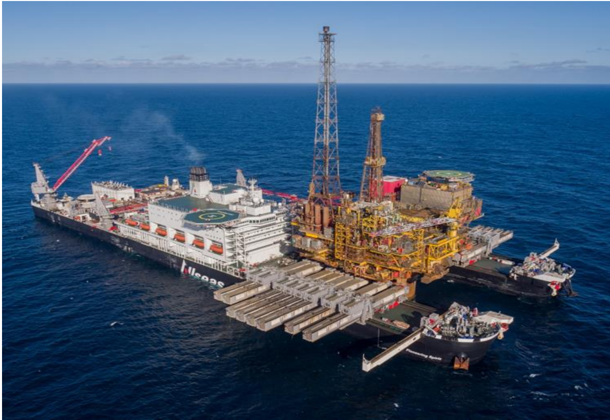
Figure 16. TLS Beams Extending from both Hulls of the Pioneering Spirit , Brent Delta, April 2017.
