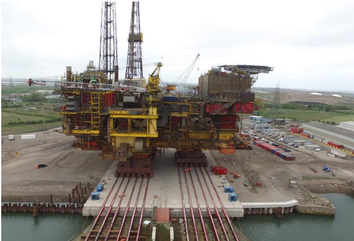
Figure 30. Brent Delta Topside Skidded onto Quay 6 ASP Facility Teesside, May 2017.
