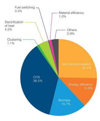
**Figure 4.1** 2015 analysis on the technical potential for emissions reduction in 8 most heat-intensive industrial sectors Source: BEIS, 2015.
