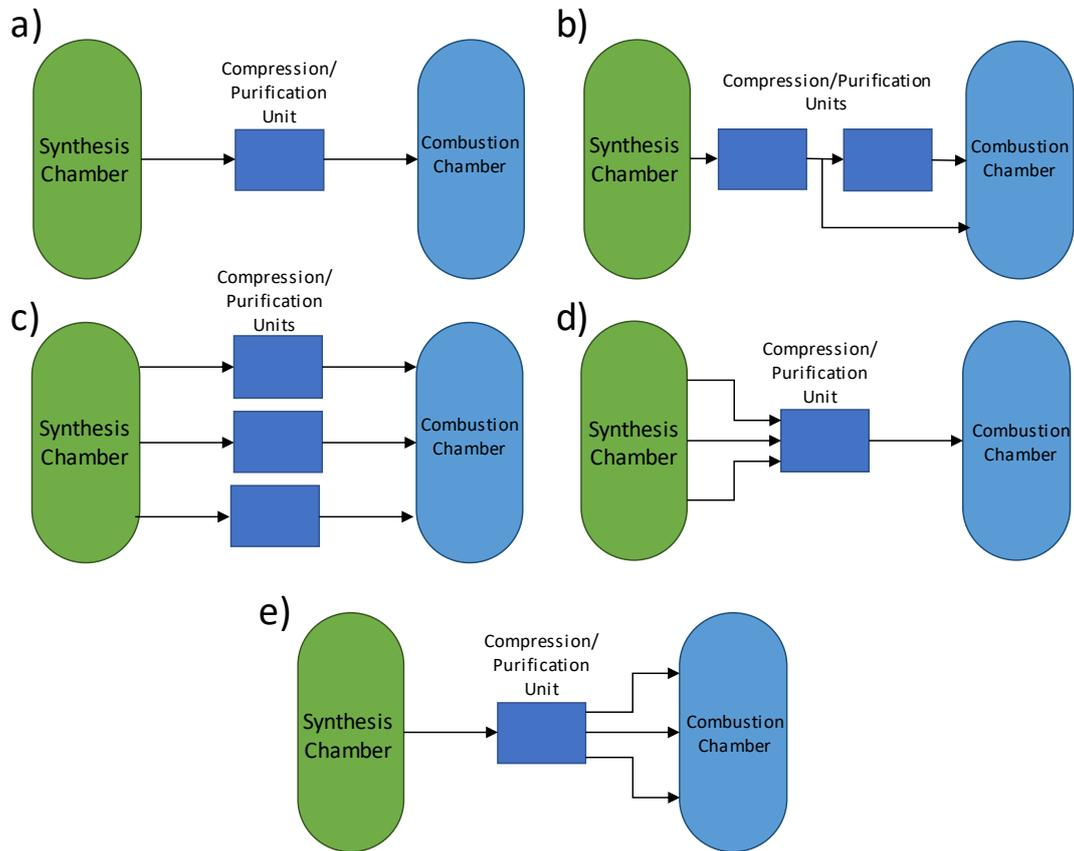
Figure 2. Examples of non-compliant configurations. The lines in red show paths where the *Advanced Fuel* does not pass through the *Compression Unit(s)* or *Purification Unit(s)* when being transported from the *Synthesis Chamber* to the *Combustion Chamber*
