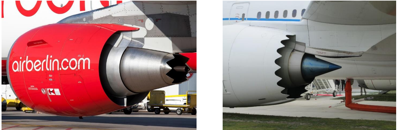
Figure 6. Left: core chevrons on a A321 (from pprune.org ). Right: fan chevrons on a B787 (Personal photo).
