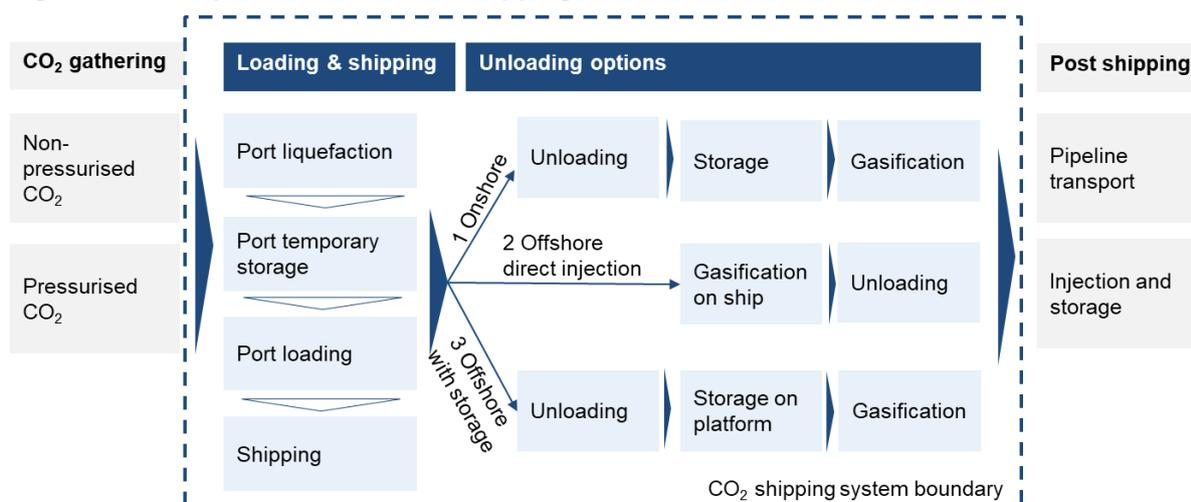
Figure 3-1 shows the components of the CO<sub>2</sub> shipping chain which are in the scope of the model. CO<sub>2</sub> is liquefied after arriving at the liquefaction plant in either pressurised or non-pressurised form. It is stored in liquified form in temporary storage tanks. From the tanks it is loaded onto the CO<sub>2</sub> carrying ship via a cargo handling system and then transported by ship to the destination.
