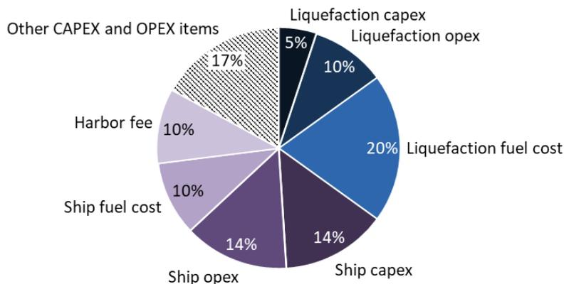
Figure 5-2 Costs components of CO<sub>2</sub> shipping for the central case (£/tCO<sub>2</sub>)
