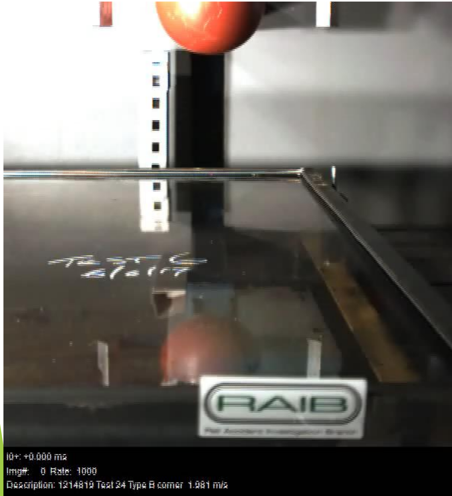
Headform test - 210mm above window (corner)
