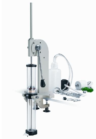
**Figure AA4** Elution tube (standing - threaded at one end) elution base (with stainless steel tube attached) concentrator tube (laying - threaded at both ends) and concentrator base (with tap)
