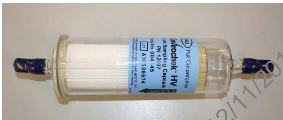
Attach the filter capsule to the water supply under investigation, ensuring that the direction of water flow is as indicated on the capsule. It may be appropriate to flush or retain any residual debris from the sampling tap or pipe before it is connected to the filter housing. This will depend on whether the debris needs analysing, or whether the debris is to be analysed with the water to be filtered.
