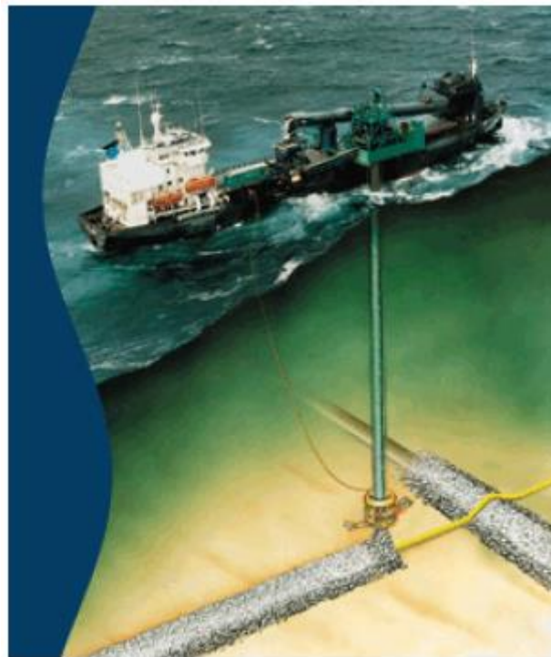
Figure 4-3 – Remedial Rock Cover Installation Illustration
