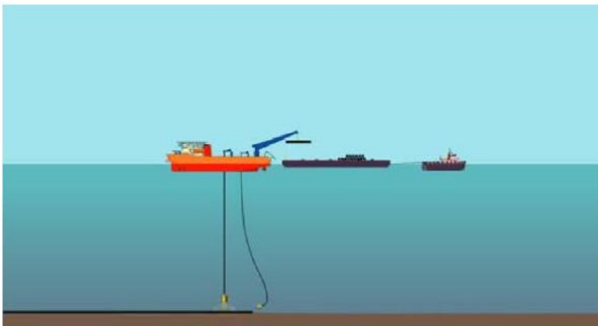
Figure 4-1 – Cut and Lift Pipeline Removal Illustration
