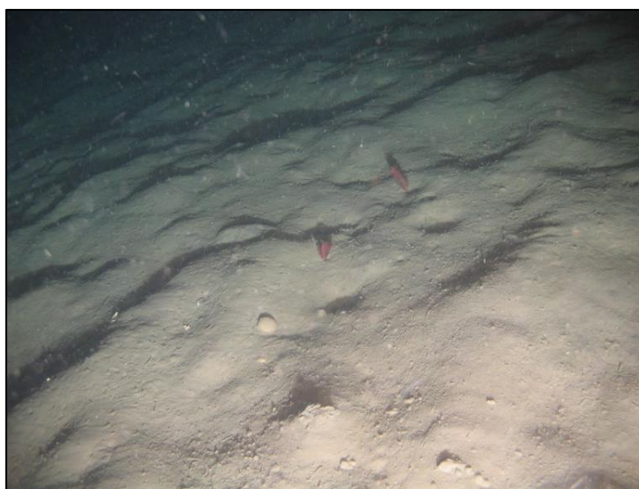
Figure 2-4 Camera still showing the silty fine sand seabed sediments in the area of the Goldeneye platform (Fugro, 2010).
