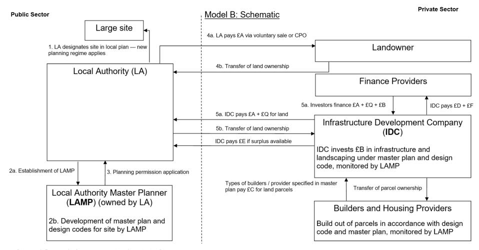
Stages 1-5 occur before any construction starts. Stages 4 and 5 occur simultaneously to avoid any financial exposure for the local authority. Remaining stages occur gradually as site is built out.
