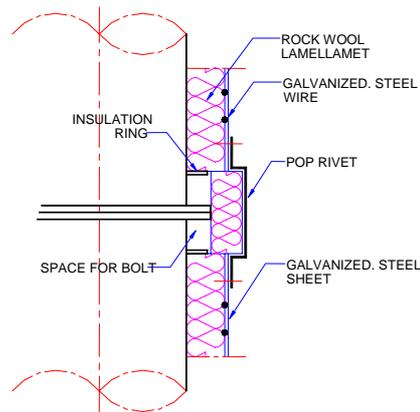
**Figure 3-4 – Insulation method on flanged part**
