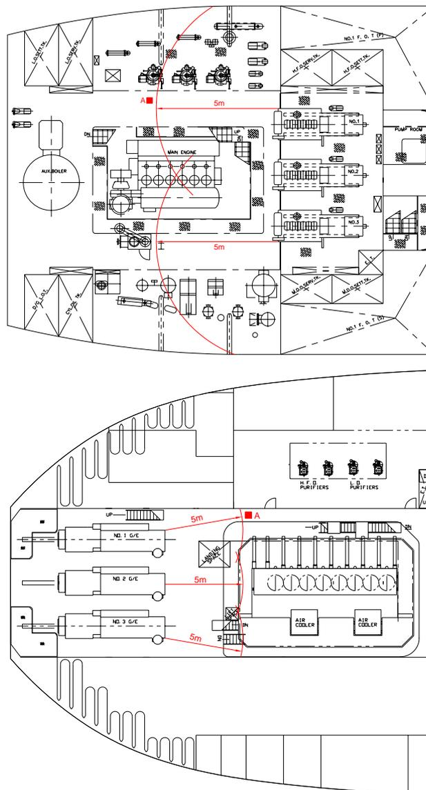
Figure 3-9 – Isolation valves arrangement for multi-engines
