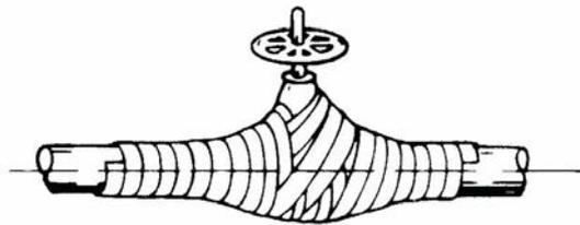
**Figure 3-1 – Example of correct taping method**
