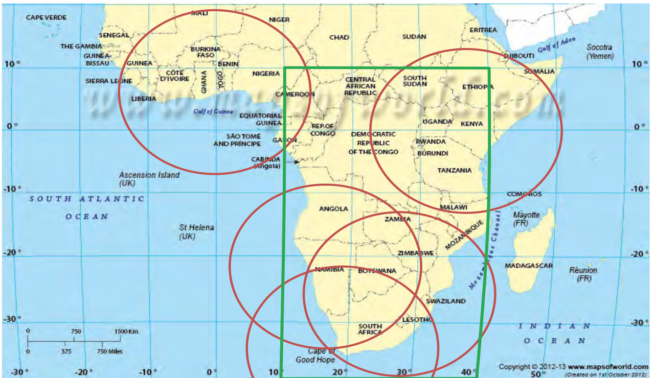
Figure 13: Ground station coverage and FireSat area of interest
