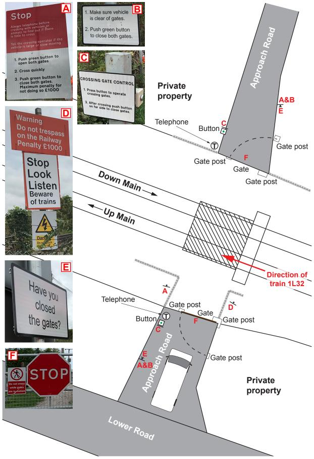
Figure 4: Frognal Farm crossing layout showing signage placement and approximate stopping location of the van
