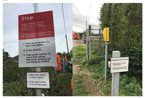
The signs at Frognal Farm crossing, showing the instructions to vehicle users (left) and the telephone cabinet, gate operating button and subsidiary instruction sign (right)<sup>13</sup>
