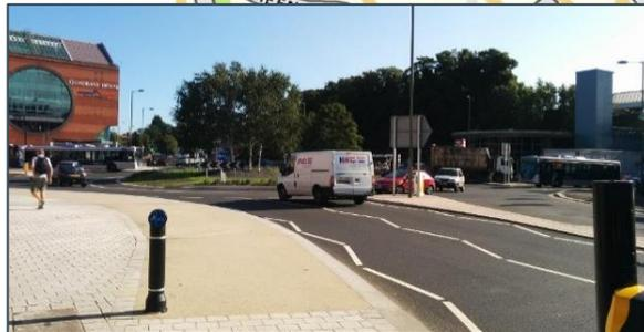
One-way system changed to two way operation. Carriageway narrowed to allow paths to be widened. Continuous shared pedestrian and cycleway provided around the town centre.
