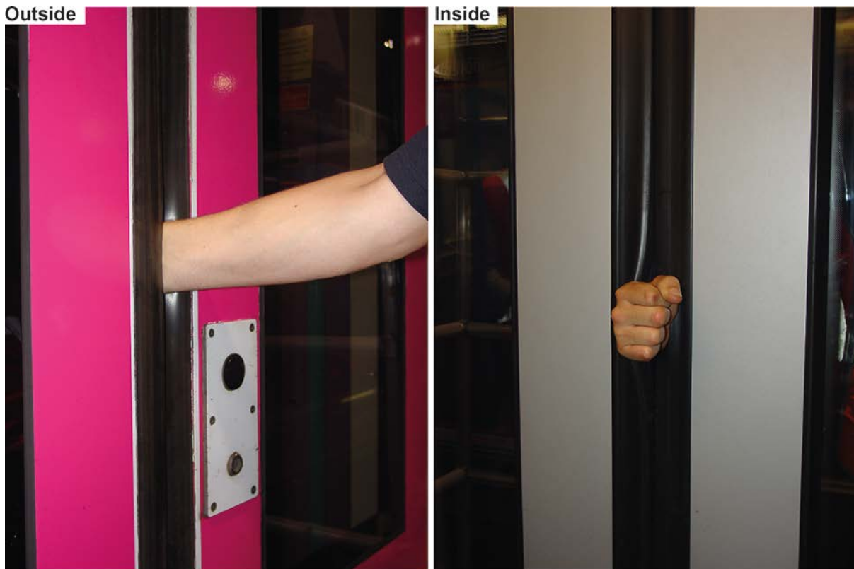
Adult male wrist, approximately 45 mm by 70 mm, trapped in a class 185 door (of similar design to a class 350 door) detected as closed and locked
