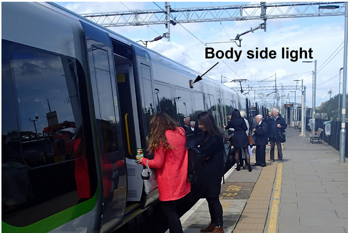
Body side light - not illuminated when doors are detected as closed and locked
