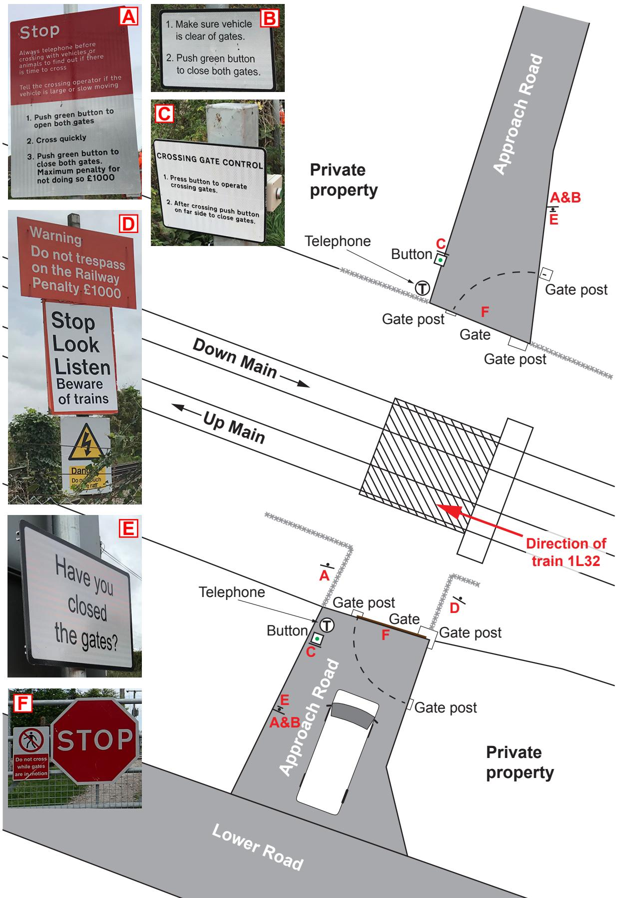
Figure 4: Frogna Farm crossing layout showing signage placement and approximate stopping location of the van
