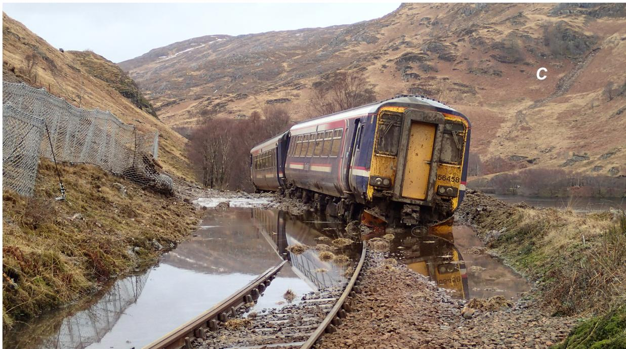
Figure 3: Front view of derailed train. Another recent landslide is visible in the distance on the opposite side of Loch Eilt (marked 'C').
