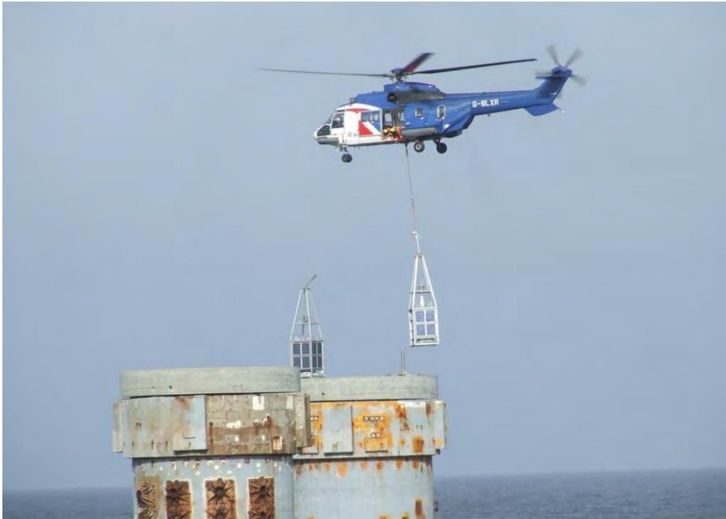
**Figure 2.17 AtoN unit deployment by helicopter**
