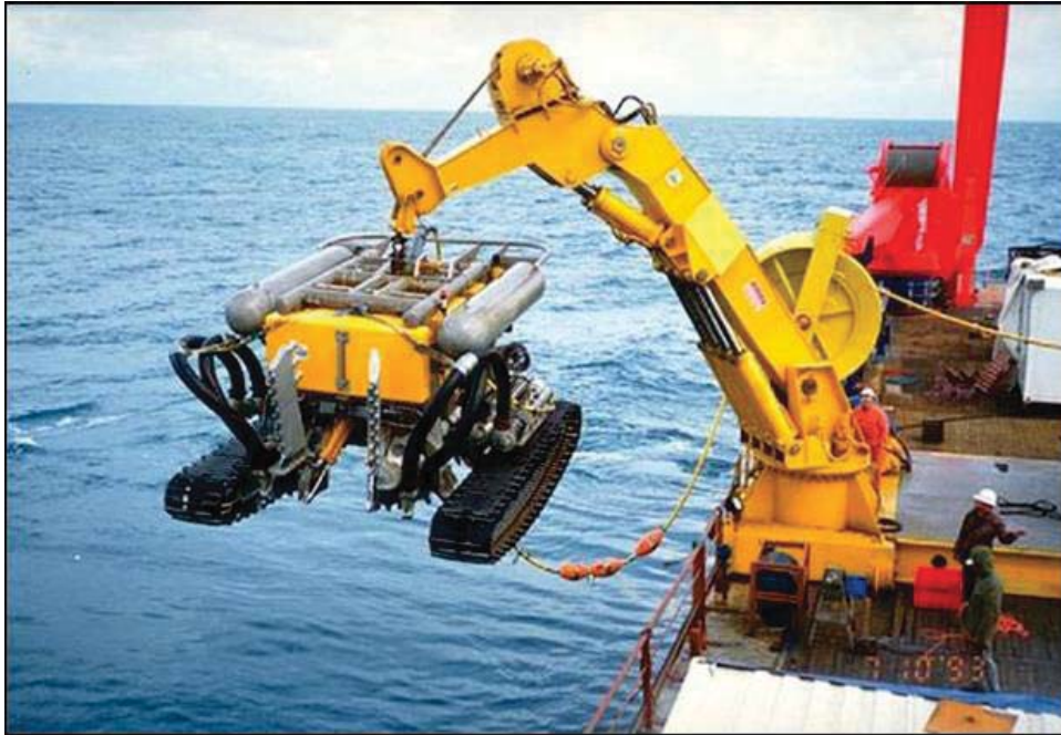
Figure 3-9: Example of a trenching / jetting unit that could be used.
