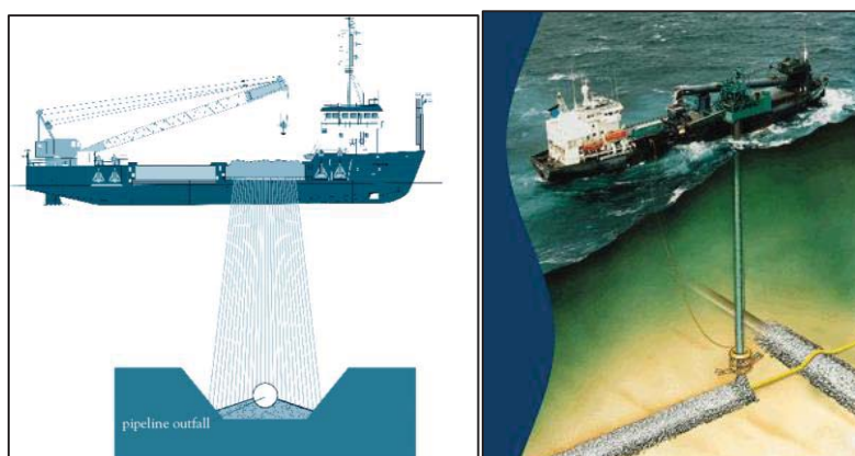
Side Stone Dumping Vessel / Fall Pipe Vessel
