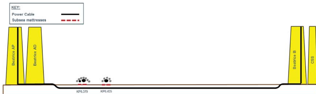
Figure 15 PL4330 - Beatrice AP to Beatrice B Power Cable Illustration
