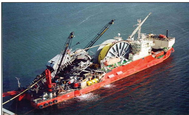
Reel lay vessel
