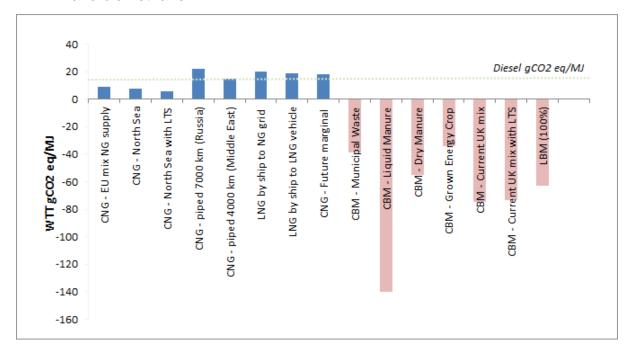
5.8 It is important to consider the impact of well to tank emissions as well as the tank to wheel emissions in order to be clear about the overall (well to wheel) emissions associated with using gas in HGVs instead of or as well as diesel.
