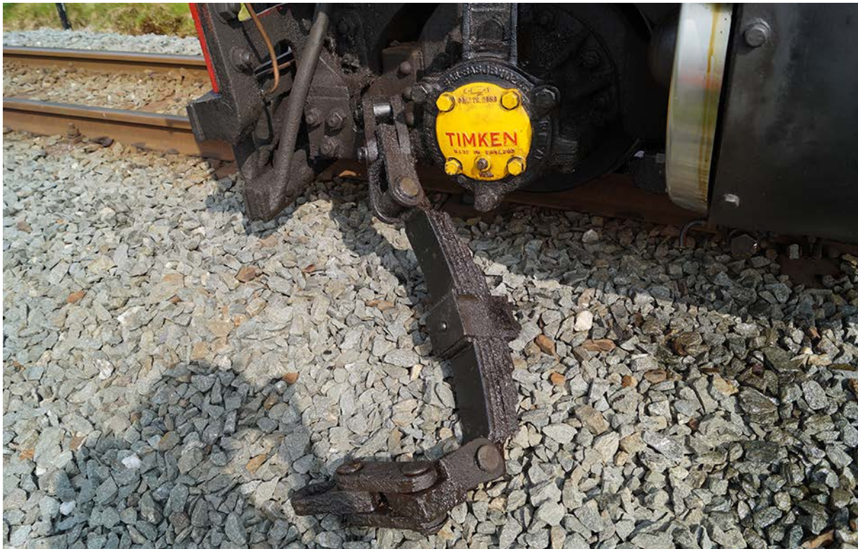
The derailed leading wheelset. The leaf spring suspension and associated components had become disarranged as a consequence of the failure (photograph courtesy of Ffestiniog and Welsh Highland Railways).
