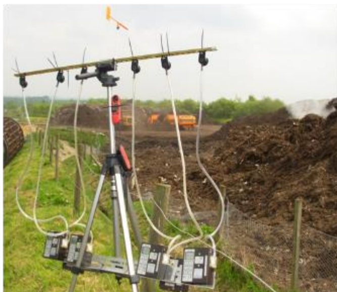
Figure 5.5 IOM Sampling heads in the field (note the sampling heads are fixed to bar to maintain the correct orientation)
