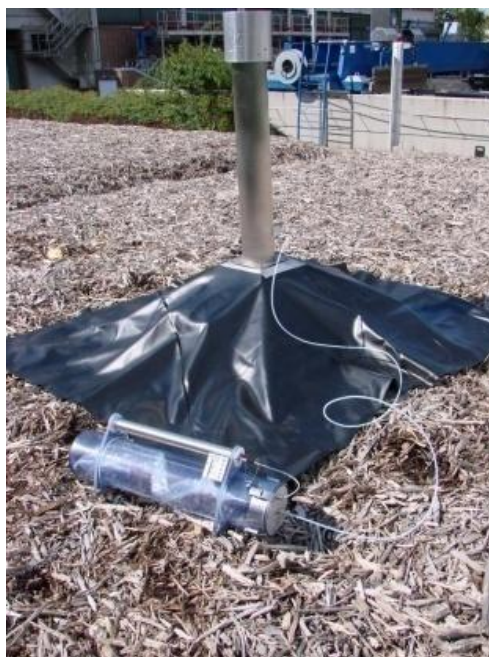
Figure 4.2: Sample hood for measurement of flow velocities and for sampling biofilters (the hood can also be used to measure odour, as seen in this figure)
