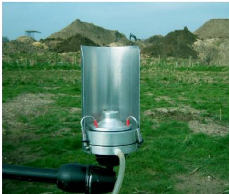
Photograph 5.1: Single stage impactation sampler (Andersen) set up in the field
