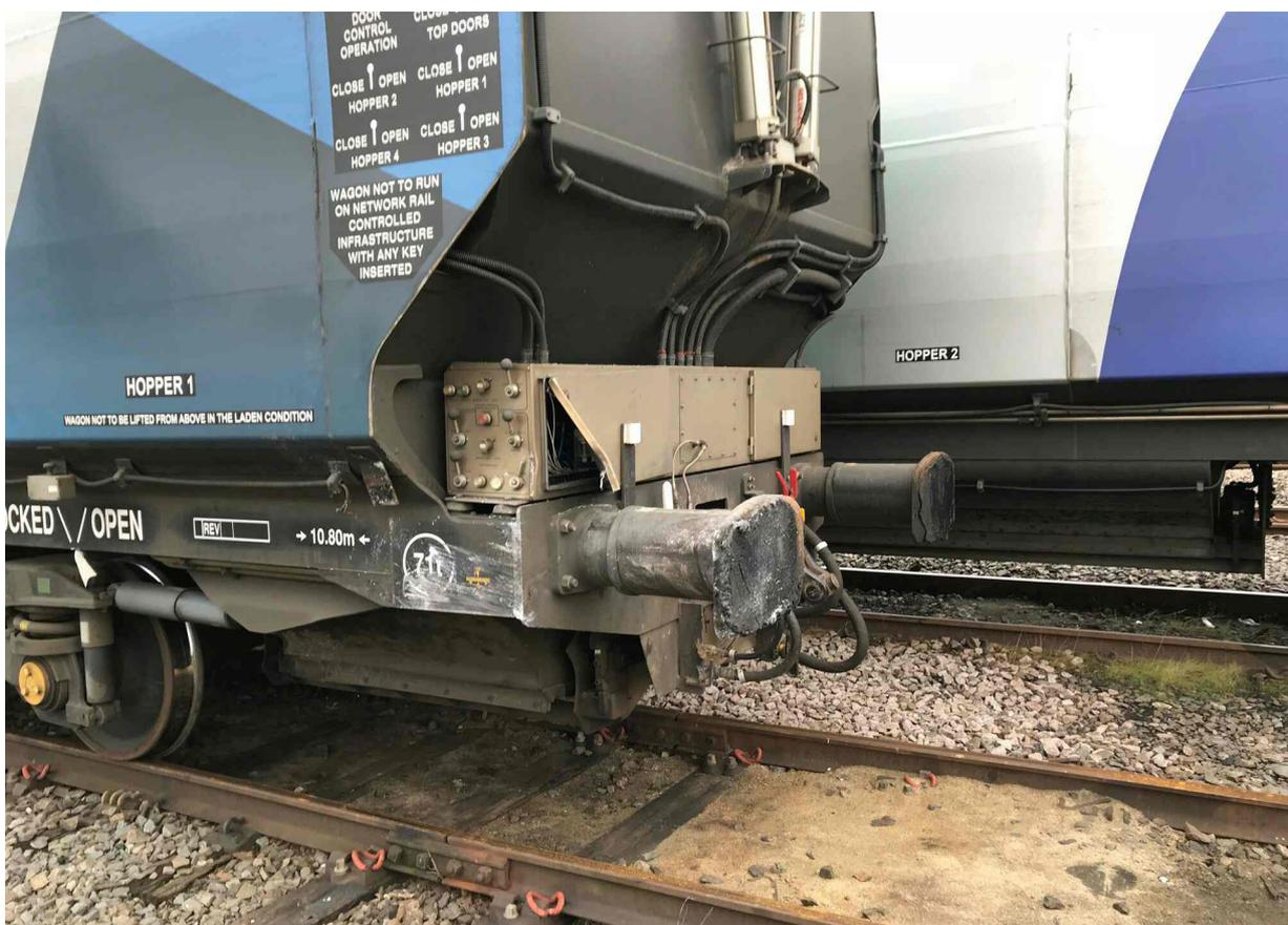
Figure 7: The damage sustained by the rearmost wagon as a result of the accident (image courtesy of Network Rail)
