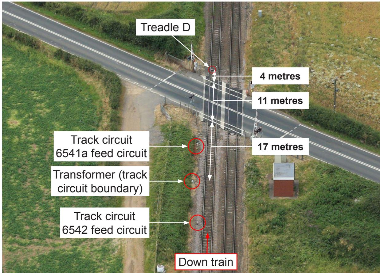
Figure 11: The track circuit and treadle arrangement at Stainforth Road AHB (underlying image courtesy of Network Rail)
