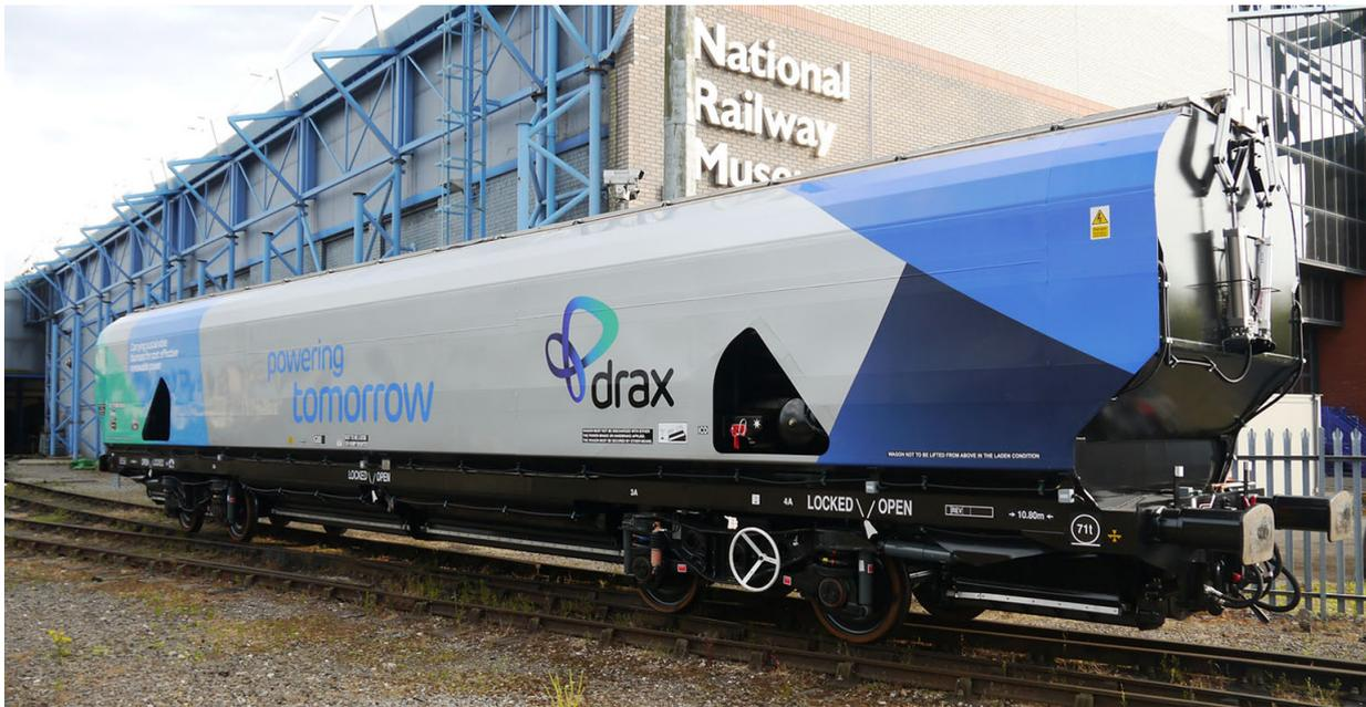
Figure 4: A library image of a type IIA Biomass wagon (image courtesy of Drax Group PLC)
