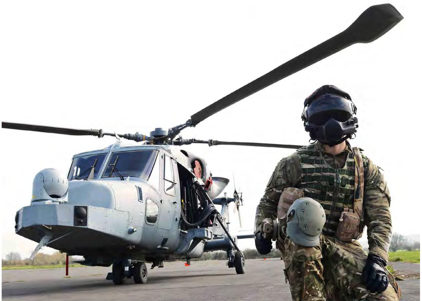
Wildcat Mk1 Helicopter fitted with 50Cal Browning M3M Machine Gun and its Door Gunner
