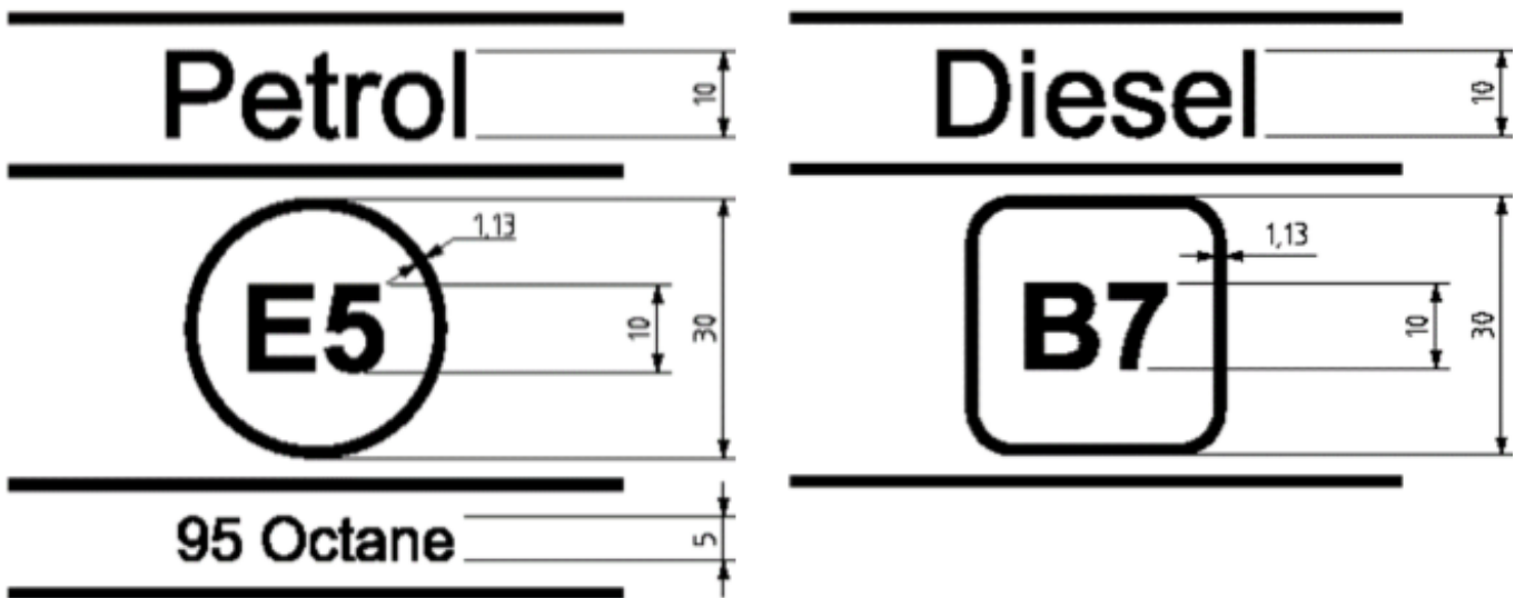
Figure 2. Fuel dispenser labels for E5 Petrol and B7 Diesel. The labels include the minimum information required.
