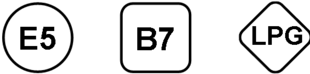
Figure 1. Graphical identifier examples for E5 petrol, B7 Diesel and LPG.
